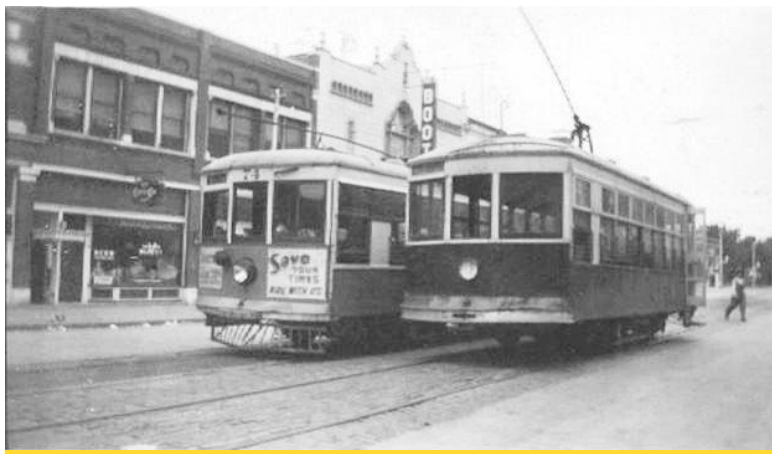
No.# 74 - American Car Co. (1925) and No. 15 an 18' Birney in one of the city operations - probably part of a 25 car order originally built by Osgood Bradley for a Rhode Island line.
