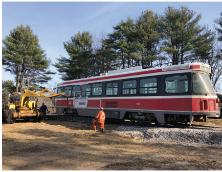
Above: A Pettibone Speedswing is used to shift CLRV 4068 on temporary Toronto gauge track. KO
