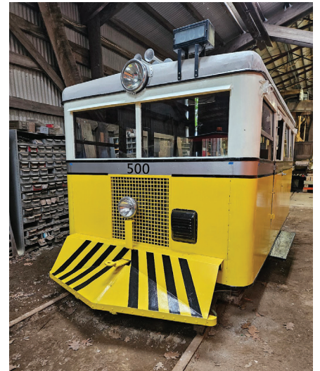
Above: The body of Bay State 4175 rests on blocking to allow the trucks to be rolled under the car. DR Above right: Our bus from Iowa has been brightly painted by volunteers with shop staff help. KO Right: B&M gasoline motor car 500 is now ready for rescue missions if trolley power fails. KO
