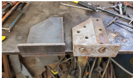
Above: New transom gusset plates being fabricated for Dallas 434's trucks.
