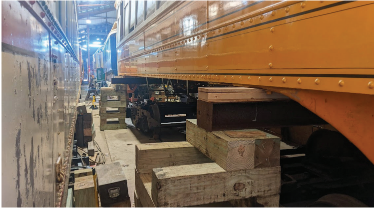
Above: The body of Bay State 4175 rests on blocking to allow the trucks to be rolled under the car. DR Above right: Our bus from Iowa has been brightly painted by volunteers with shop staff help. KO Right: B&M gasoline motor car 500 is now ready for rescue missions if trolley power fails. KO
