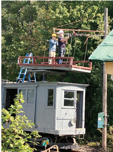
Above: Old and new wire technology contrasted. On the left a 125 year old platform raises and rotates and carries two. At right a road/rail capable bucket truck has wide multidirectional reach. RD
