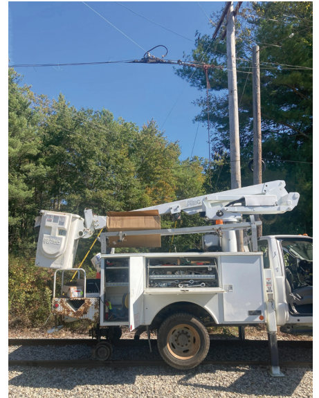
Above: Old and new wire technology contrasted. On the left a 125 year old platform raises and rotates and carries two. At right a road/rail capable bucket truck has wide multidirectional reach. RD
