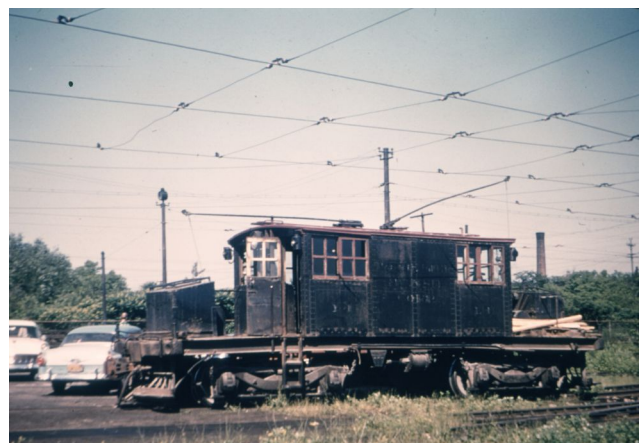
A home-made locomotive at Rochester produced by the company's shops from GE kit in 1928
