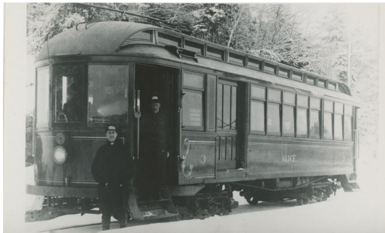
Double truck closed combination car No. 3 - the Alice - (John Stephenson Car Co. - 1902)
