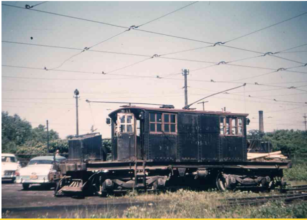
A home-made locomotive produced by the company's shops from GE kit in 1928
