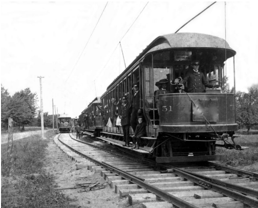
No. #51 & #50-Ottawa Car Co, (1900) It appears that circa 1915 opens were banned in a major city on the system due to accidents involving running boards - they were either rebuilt or transferred.
