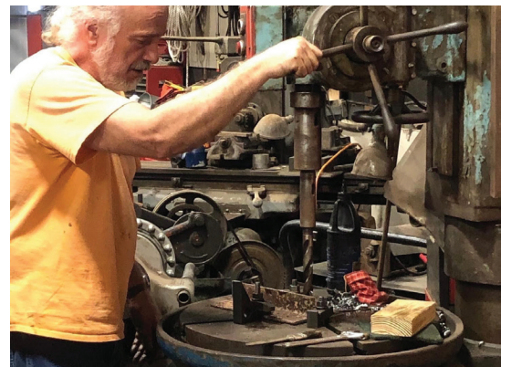
James van Bokkelen fabricates a rail joint component.
