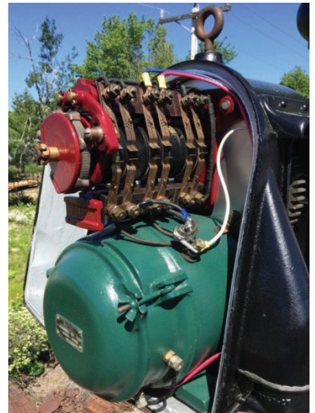
A completely rebuilt signal mechanism ready for installation and operation of a signal arm. DD
