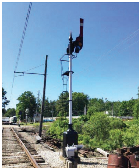
A rebuilt semaphore approaching McKay crossing.
