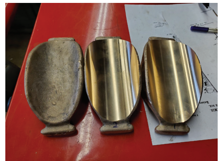
Newly cast and machined motor axle bearings for the Narcissus . DR
