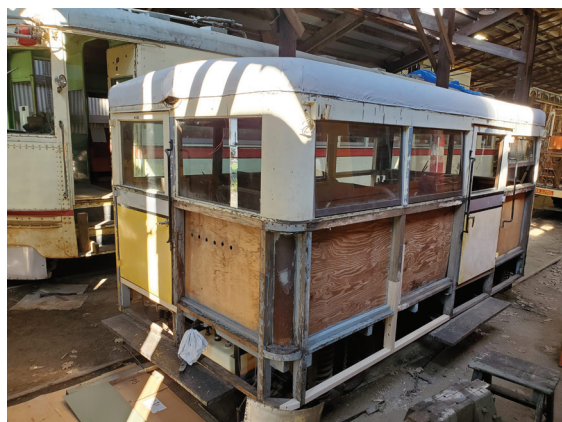
Boston & Maine inspection car 500 awaits new side panels. KO
