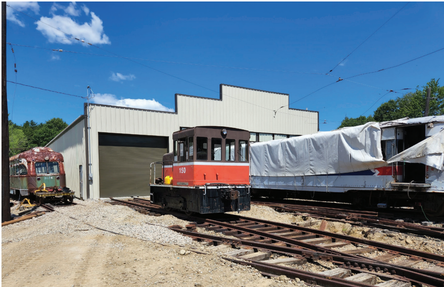
Locomotive 150 rests on the newly rebuilt track that feeds the expanded area of Fairview Carhouse. KO
