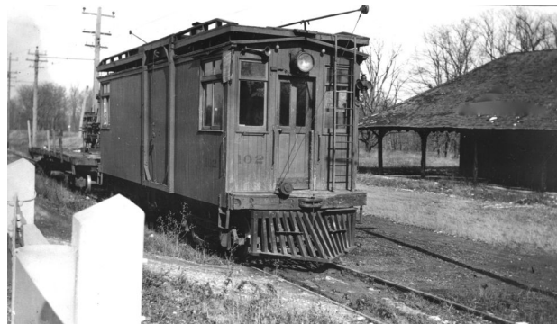
#102 Line Car and Plow dismantling the line in 1933. This car was apparently saved along with the 3 freight motors for service on the spur to the generating station.
