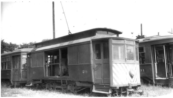
#29 built by St. Louis Car Co. (1899) on a design by Ford, Bacon & Davis. Converted to a rail grinder and then sand car. Ultimately restored in its sand car
