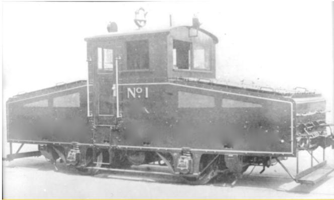
# 1 - Battery locomotive - built by Atlas Car & Manufacturing Co. (1926). Assigned to a power plant moving coal gondolas over a distance of some two blocks.
