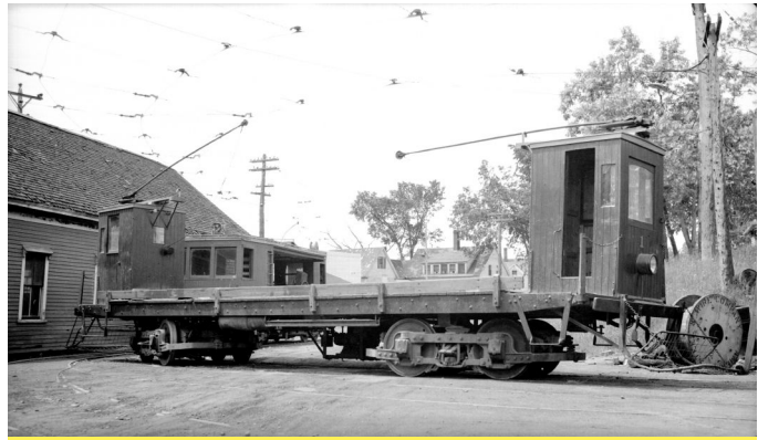
41 ft. double cab motor flat No. # 1 - company shops (former 14 bench open)
