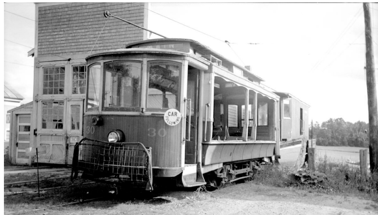
#30, built by Brill, after conversion to a sand car from a second-hand closed car obtained from an adjacent railway in 1927. The car is at the carhouse located in the same town as the initial postcard image.
