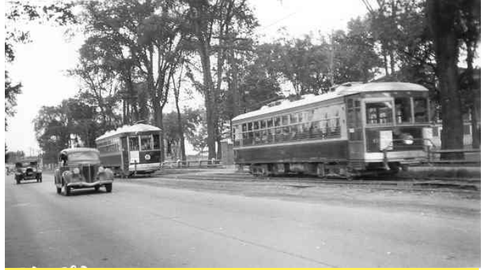
No. #60, 31 ft. safety car - JG Brill (1922) acquired 1931 passing No. 50, 33 ft. closed car - Kuhlman (1918) in namesake city
