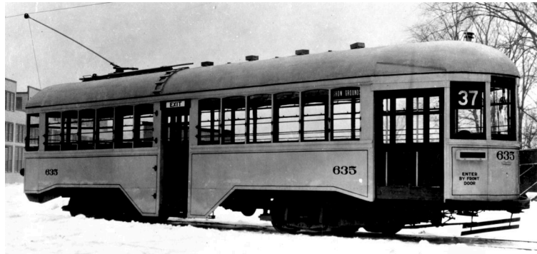
Steel PAYE car #635 - Kuhlman (1916) Coupler added in 1917 to haul trailers
