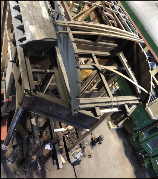
Major structural work to the car's vestibules has begun. Seashore Trolley Museum collection
