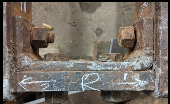
From top to bottom: #1 truck partially disassembled; detail of bolster cracks; cracked end frame, right side; "re-made" gusset plate; repairs on the transom brace, indicated bolt was loose. BT
