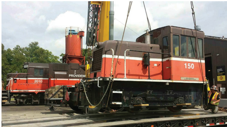
Above: A generous donation enabled acquiring Providence & Worcester diesel 150 for use as a shifting and rescue locomotive. Here a crane loads the diesel for the trip to Maine. TL Right: The crane just after unloading in May JS Above right: Loco 150 on Seashore rails. KO
