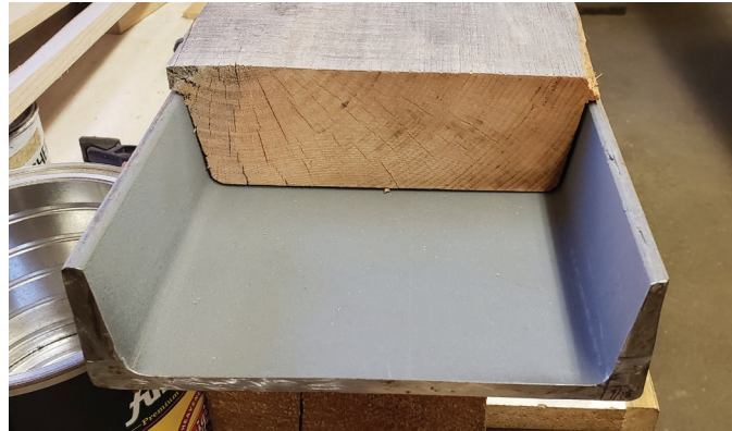
The Narcissus ' composite wood-steel side sills take shape.
