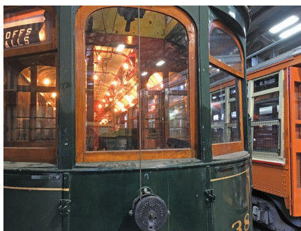
Above Left and Right: The second car acquired by the Museum was Manchester 38 in 1940. Built in 1906 by the Laconia Car Company, the car represents the highest level of wood craftsmanship. The bare filament bulbs make the varnished cherry glisten. Rewiring the lights was completed in 2019. RD
