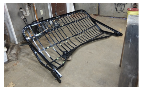
Top: Reproduction of fenders like those on 4188 for Bay State 4175 has made great progress. Middle: Donald Curry heats rivets for Heidi Schweizer to drive with a pneumatic gun. Lower: The second fender nearly complete. DC
