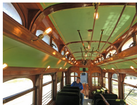
Above Left and Right: The second car acquired by the Museum was Manchester 38 in 1940. Built in 1906 by the Laconia Car Company, the car represents the highest level of wood craftsmanship. The bare filament bulbs make the varnished cherry glisten. Rewiring the lights was completed in 2019. RD
