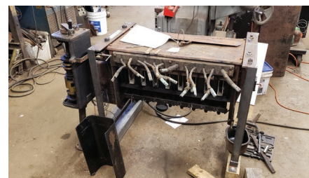
An authentic Westinghouse HL control system for the car was located in Seashore's parts supply, including master controllers ( left ) and the underfloor switch group ( above ). Both are being overhauled by project staff. PM
