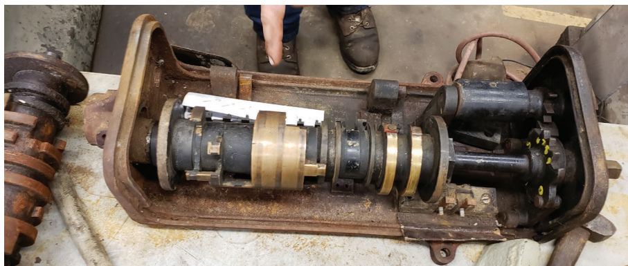
An authentic Westinghouse HL control system for the car was located in Seashore's parts supply, including master controllers ( left ) and the underfloor switch group ( above ). Both are being overhauled by project staff. PM
