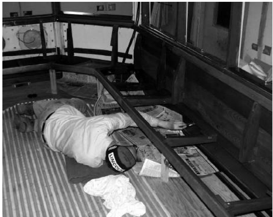
Below: Volunteer Amy Litchfield treats a window post on Connecticut Company 1160 in preparation for yellow and white finish colors. JS
