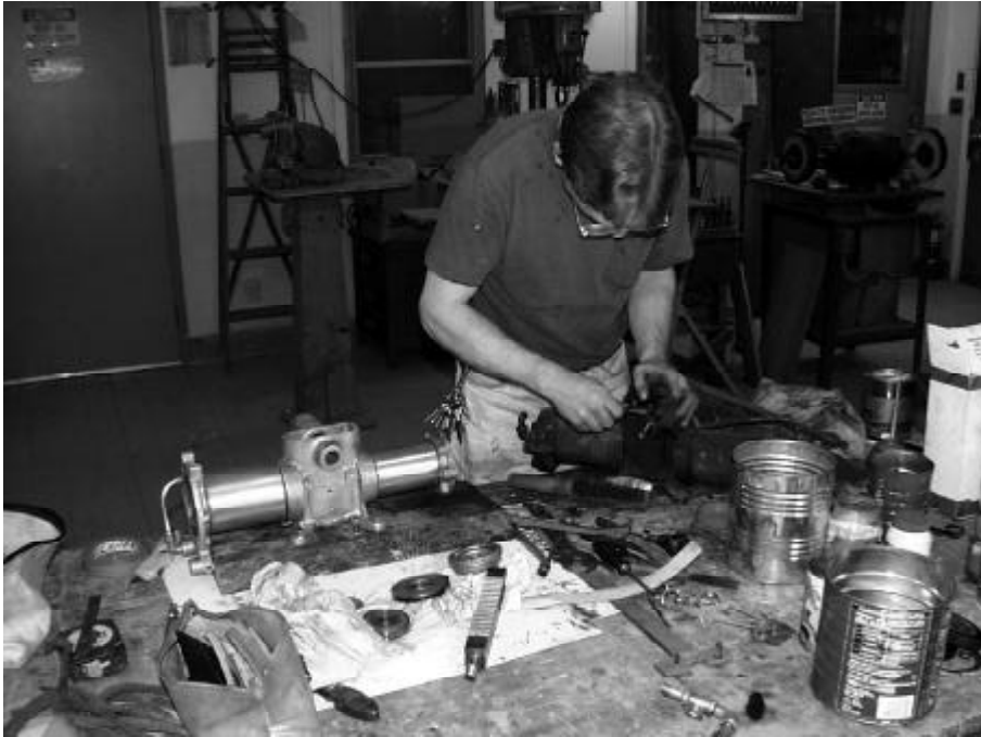
Above: Project sponsor Conrad Misek makes repairs to a door engine from one of the Museum's two Philadelphia-Camden bridge subway cars. The cars, of a distinctive art deco design, symbolize the heavy duty equipment put into service on big city rapid transit systems in the 1920s and 1930s. JS
