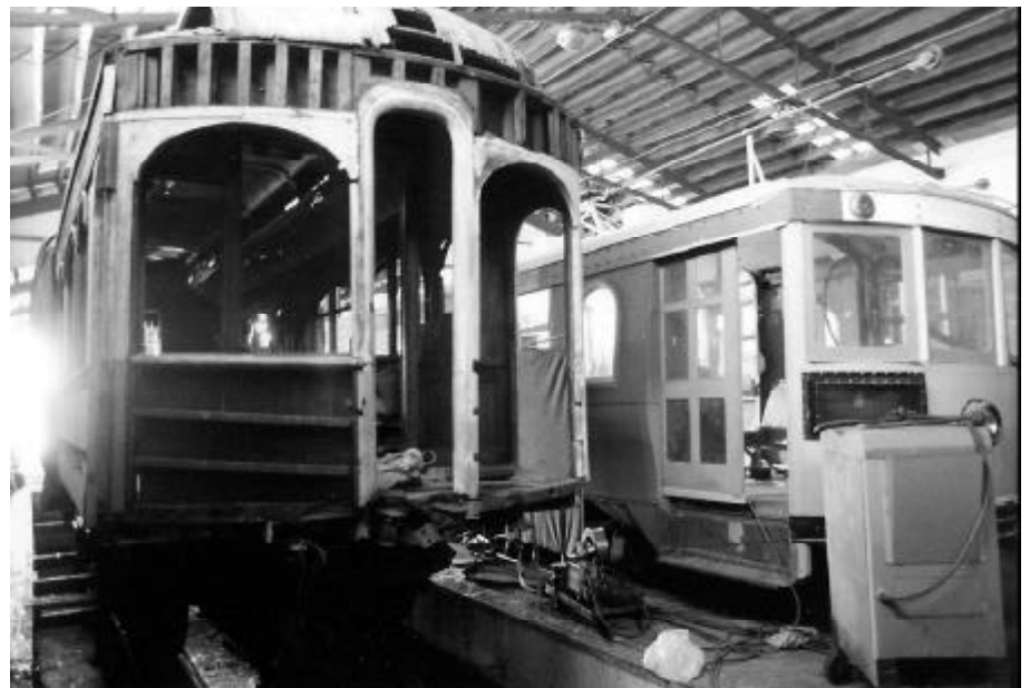
Below: Two of the major restoration projects underway in the shop, Portland-Lewiston interurban car The Narcissus and Wheeling Curved-side 639, rest on adjacent tracks. An extensive research phase has started on The Narcissus in preparation for completing rebuilding of major structural parts. DC
