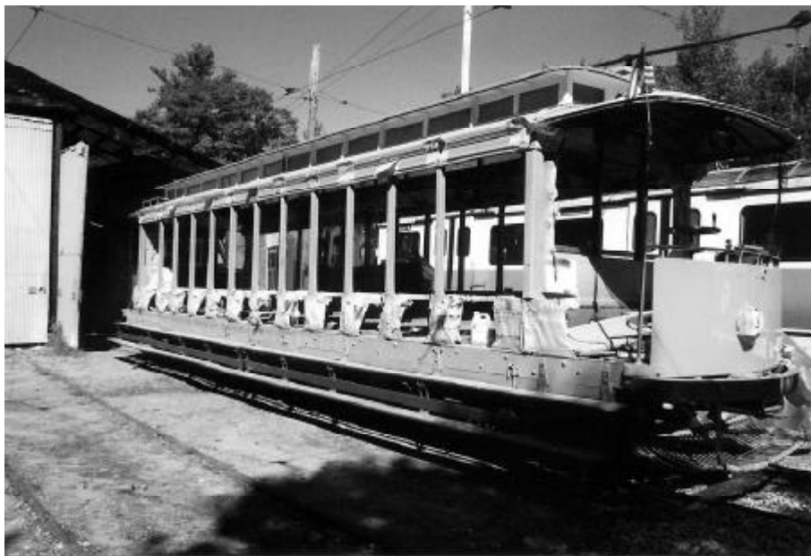
Above: The Museum's New Haven open cars—three active and one unrestored—have been the backbone of the public operation for 45 years. The result is a periodic need for restoration. Brill-built 303, arguably the most rugged of the four, is in the midst of a very careful overhaul and refinishing. DC
