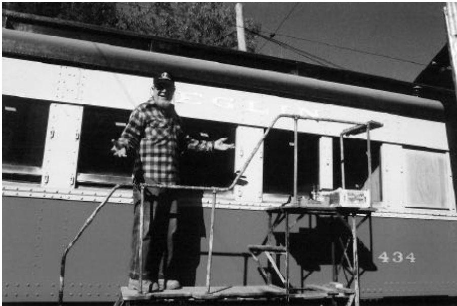
Above: The restoration of steel interurban car 434 from the Chicago, Aurora & Elgin continues to make rapid progress. Here longtime volunteer Jean Deschenes takes a break from applying the lettering to the light blue/gray letterboard. The sides are red in the 1951 livery being applied to the car. DC
