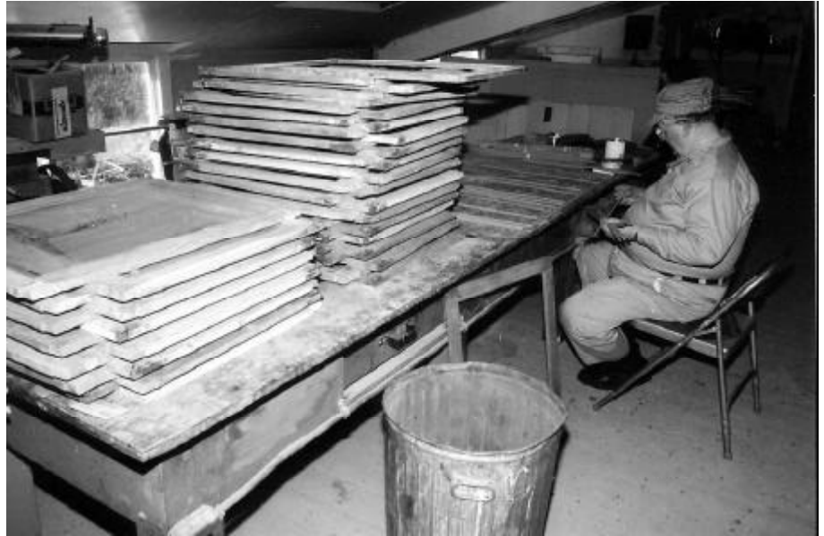
Above: Ron Newton spends a late fall afternoon working on the daunting stack of window sash from Eastern Massachusetts Street Railway semiconvertible car 4387. As the car features multiple piece sash that slide completely out of sight there are many pieces to treat when repainting is needed. DC
