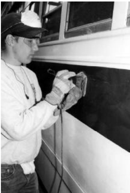
Below: Phil Dominguez prepares a section of the blue paint on Southeastern Pennsylvania Transportation Authority PCC car 2709. DC
