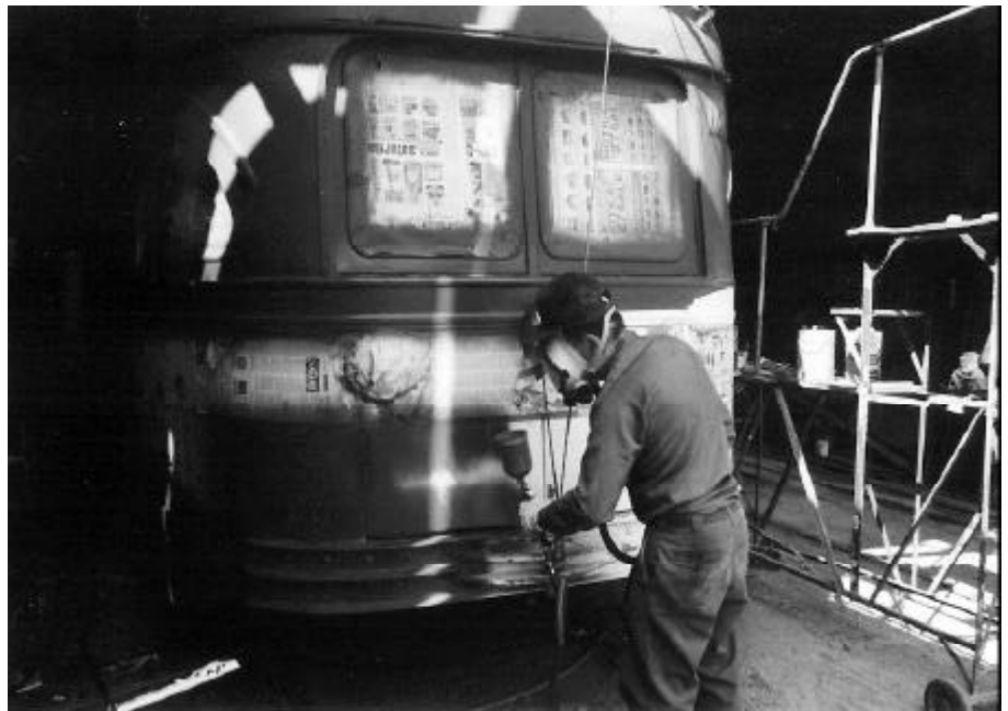
Below: Donald Curry sprays primer onto 2709 as a partial repainting of the car is underway. Interestingly, other members of this 1948-built series of cars run regularly on San Francisco's Market Street and still others are about to be restored for service on Route 15 Girard in their native Philadelphia. DC
