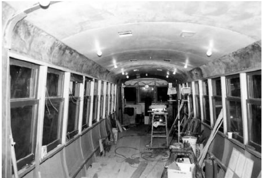
Above: The long-running restoration of Wheeling, WV Curved-side car No. 639 made considerable progress this year. The car's interior now features a completed floor, cork insulation along the sides, a full set of advertising card racks, new headlining, extensive wiring, and much newly fabricated interior trip woodwork. The car will be one of the most extensively rebuilt cars at Seashore. DC
