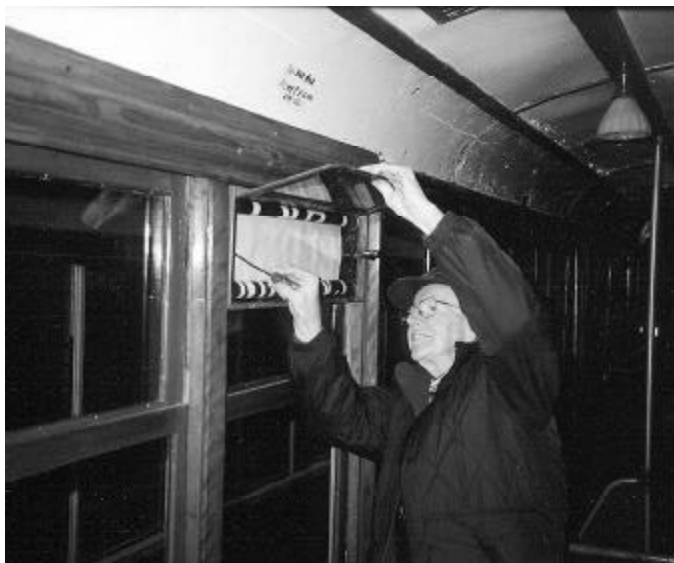
Above: Ken Haselton installs a destination side in one of the side sign boxes on Toronto Peter Witt 2890. The car came in a trade with our Canadian friends at the Ontario Electric Railway Historical Association in 1999.
