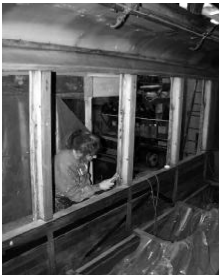
Below: Volunteer Amy Litchfield treats a window post on Connecticut Company 1160 in preparation for yellow and white finish colors. JS
