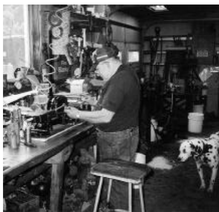
Below: Veteran shop machinist Ed Johnson, with Jake watching, puts the finishing touches on his final project at Seashore, complete rebuilding of a sliding door engine for Wheeling 639. FM
