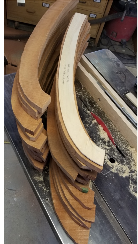
Above: Expert woodworker Lary Shaffer fabricates replacement window frames for the car's arched stained glass windows. On the left he cuts the basic shape from wide mahogany boards. The resulting pieces, at the right, will be finished to the exact curve to match the glass and the car's frame. PM
