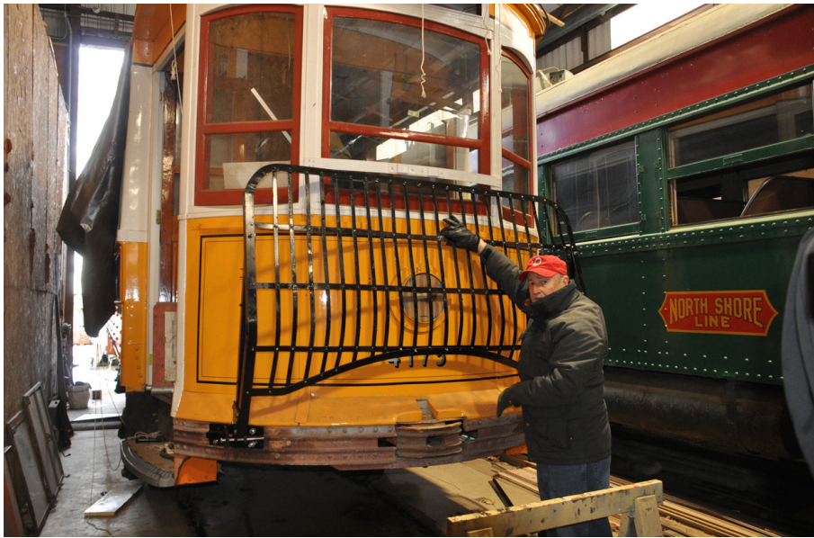
Above: Considerable effort has been expended to recreate, from photographs, the distinctive Bay State fender once carried by Bay State No. 4175. Here the newly fabricated and riveted fender is shown in the raised position. The correct suspension and dropping mechanism remain to be made. DC
