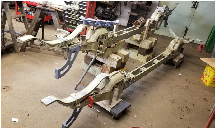
Above: Components for the truck to be placed under Lexington & Boston box car No. 4 continue to take shape, after the exact truck needed was recovered from a swamp. Here new side frame components are being assembled. DC
