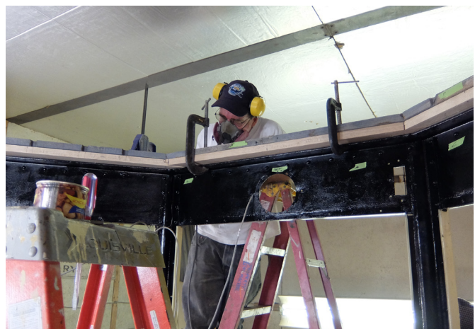
Above: Shop staff member Ernie Eaton works on the same plate at the other end of the car. The center-entrance cars, which for decades carried crowds in three car coupled sets, have a very intricate body structure. DC
