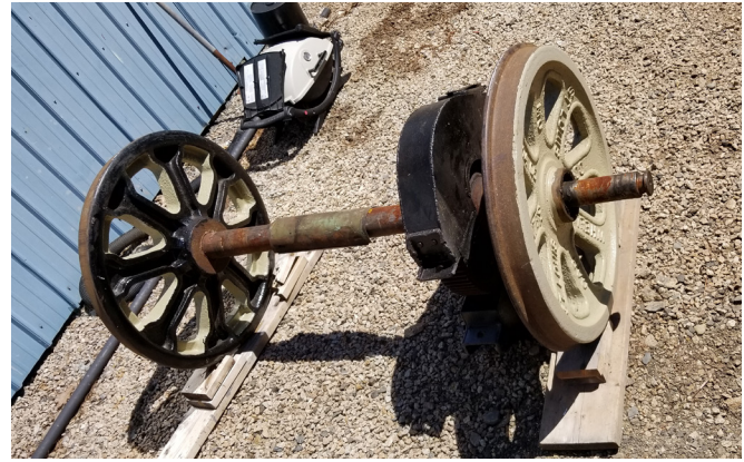
Above: A wheel and axle set from the same truck with early spoked cast iron wheels. The axles were found to be bent meaning new must be fabricated, and mounted with great care to avoid damaging the wheels. DC
