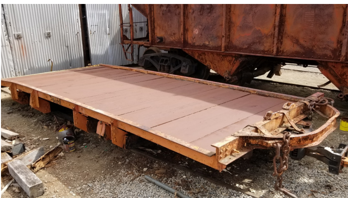
Above: This utility trailer, No. 3603 built in 1923 for the Boston Elevated Railway, remains a useful tool for transporting vehicles or equipment to sites along the main line. In 2018 its full wooden deck was replaced with thick boards. DC
