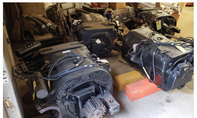
Above: Traction motors such as these from Eastern Massachusetts Street Railway No. 4387 are what powers streetcars. These have returned from AC Electric, where full preventive maintenance was performed. DC
