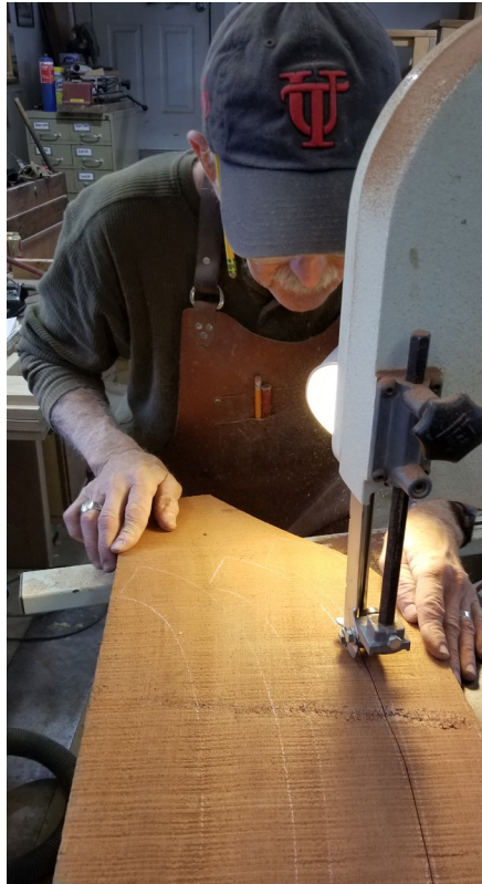
Above: Expert woodworker Lary Shaffer fabricates replacement window frames for the car's arched stained glass windows. On the left he cuts the basic shape from wide mahogany boards. The resulting pieces, at the right, will be finished to the exact curve to match the glass and the car's frame. PM
