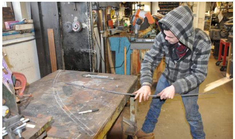
Left: Randy Leclair works on the shellacked surface of a Narcissus interior trim piece. The rich wood color is clearly coming back. DC Right: Cam Alcock bends a half-oval trim piece for Lexington & Boston St. Ry. box car 41. DC
