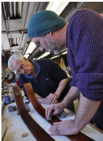
Left: Randy Leclair works on the shellacked surface of a Narcissus interior trim piece. The rich wood color is clearly coming back. DC Right: Cam Alcock bends a half-oval trim piece for Lexington & Boston St. Ry. box car 41. DC
