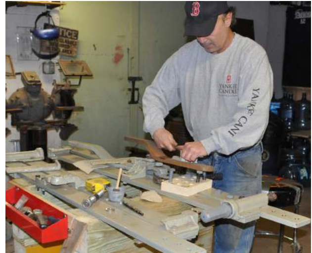
Above: John Melanson works on components for the Bemis truck being readied for Lexington & Boston 41. The truck, from a Norway & Paris (ME) car, was retrieved from a swamp some years ago! DC
