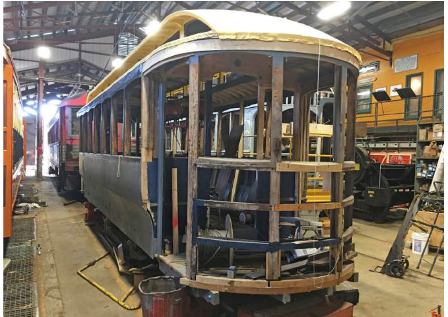
Above: The full restoration of Lexington & Boston St. Ry. single truck car 41 continues to make steady progress. Recovered as a diner in the early 1960s, the progress is striking. Three doors cut in the sides are gone; the rebuilt roof is complete; side panels are on; and truck rebuilding is well under way. DC
