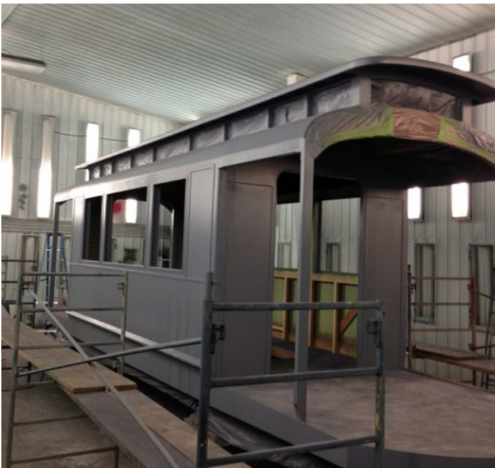
Left: The very accurate replica of parlor car City of Manchester for a private party takes shape at a Mount Desert Island boat-builder. The truck, control system, and mechanical fittings are being restored or fabricated in Seashore’s Town House Shop.
