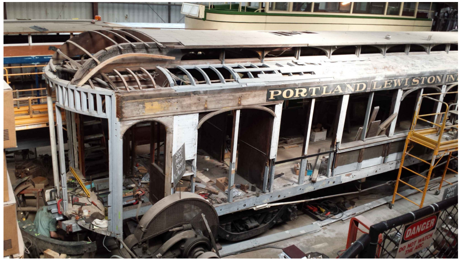
Above: After The Narcissus entered the shop, work focused on replacing corroded steel fasteners holding the wooden components together plus rebuilding the platform structural framing. JS
