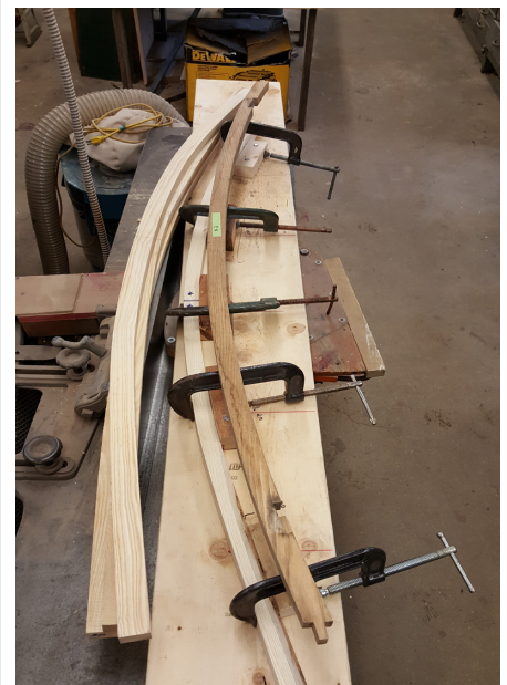
Above: Steam bending wood to make replacement roof ribs such as these for The Narcissus is an art which requires a custom jig and careful experimentation to match the original curve. PM
