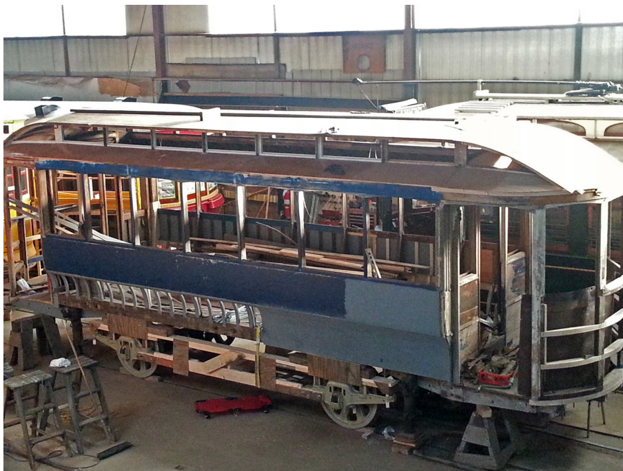
Above: Lexington and Boston No. 41 on its temporary wood-framed truck enabling it to move out of the shop during the shop roof project. Right: Volunteers Dick Avy and Jim Mackell work on the car's clerestory windows. In the background is Toronto Peter Witt No. 2890. DJ
