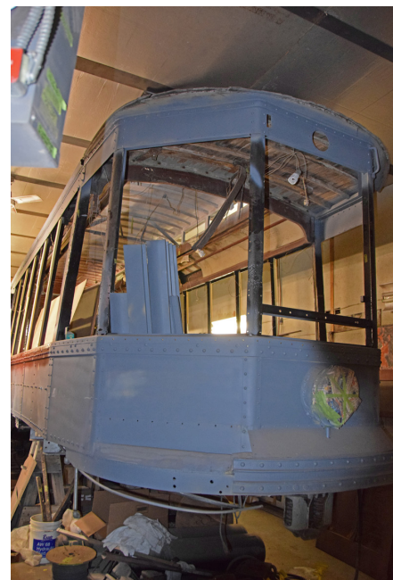
Above: At year end new donations allowed work to resume on the massive restoration of Boston Center Entrance car No. 6131. As 2016 began, efforts were focused on completing fabrication and riveting of framing surrounding the windows on both the sides and vestibule ends. JS
