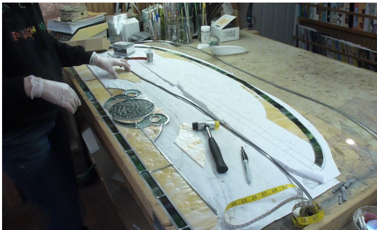
Left: Two views of the intricate work needed to rebuild the car's stained glass windows, a distinctive feature of both the side and clerestory windows.
