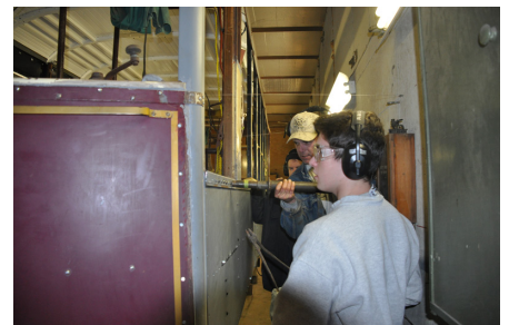
Above: Two views of hot riveting of new side panels on Denver and South Platte Birney car No. 1.
