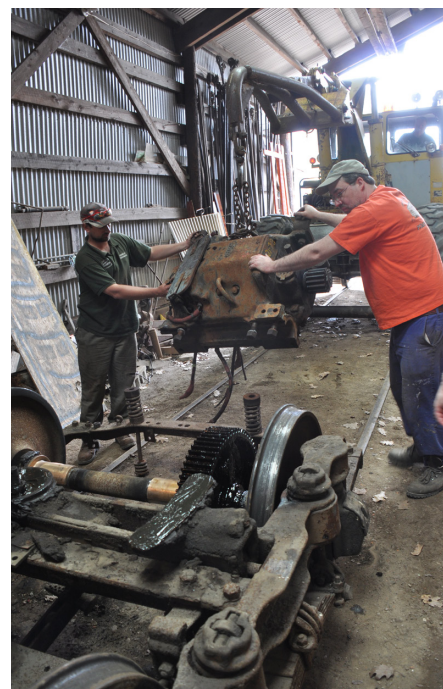
Above: Eric Gilman and Randy Leclair guide a motor for Boston No. 396 into its truck frame. This car, once used in Otto Preminger's The Cardinal is being prepared for regular operation. DC
