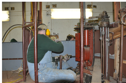
Above: Two views of hot riveting of new side panels on Denver and South Platte Birney car No. 1.
