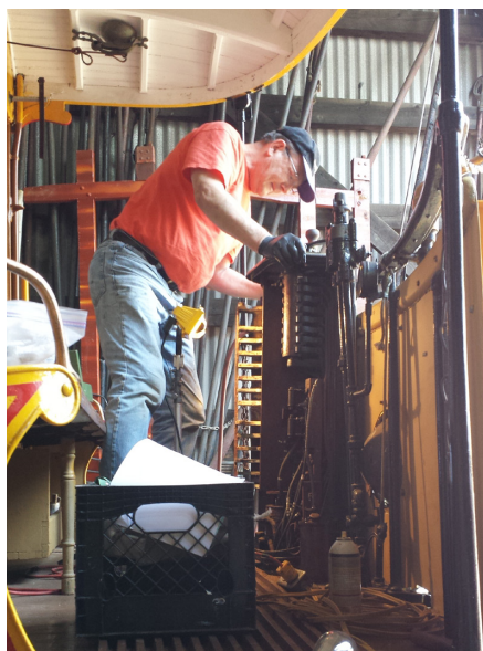
Above: Greatly increased visitorship meant much more equipment maintenance. Here Ed Dooks checks controller fingers for arcing damage. DC
