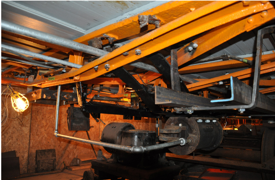
Above: Re-equipping a car that arrived as a stripped body is an arduous process involving substantial detective work plus trial-and-error. Here the brake cylinder and air compressor are being positioned under Bay State Street Railway No. 4175. Availability of replacement parts is vital to success. DC
