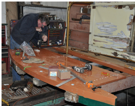
Above: Jim Mackell bores a hole in newly fabricated rear platform decking of Montreal No. 2. After 100 years the old parts had deteriorated. DC
