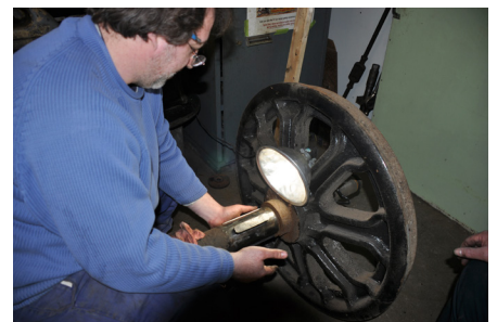
Above: Randy Leclair tests fitting of keys machined to hold the bull gear on the Bemis truck axle being adapted for use on No. 41. DC
