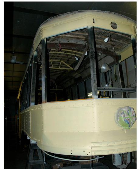
Above: Boston 6131 after completion of priming of the entire rebuilt steel body structure. DC
