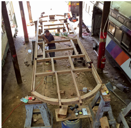
Progress in the construction of a replica of the City of Manchester parlor car for a private party: Top: The Brill 21-E truck sourced in Texas arrives. Above: The car's underframe takes shape. JS
