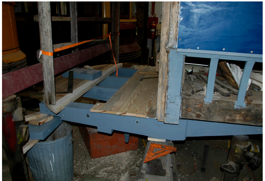
Above: Rebuilding of an end platform on Lexington & Boston Street Railway No. 41 shows progress as platform knees have been repaired or replaced as needed and new flooring is being installed. DC
