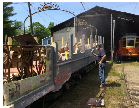
Above: Jim Mackell sprays primer on the carefully prepared and sanded exterior surfaces of No. 2, part of a complete refinishing of the car. JS
