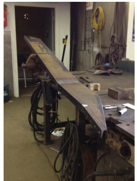
Above: A new platform knee for Eastern Mass. 7005 takes shape in the metal shop. JS
