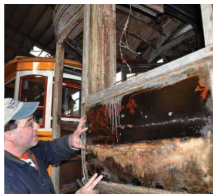
Above: Jim Mackell, Dann Chamberlin, and Dick Avy fit a new belt rail on Lexington & Boston 41, filling voids where doors had been cut in the side when it became a diner. Right: Randy Leclair examines original striping discovered during disassembly. DC
