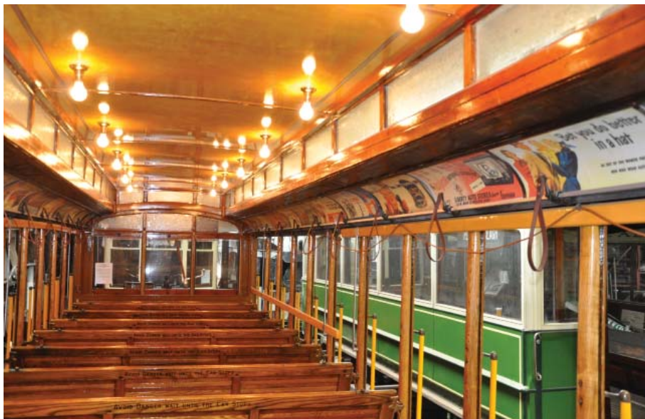
Above: Connecticut open car 838—a car in regular operation at Seashore for over a half century—glitters with new headlining and freshly varnished surfaces throughout.
