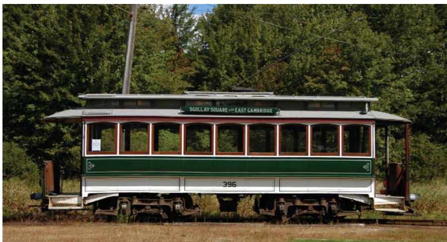
Above: Boston once had a fleet of more than 1,200 25-foot box cars such as 396. This year the car was largely repainted after completion of repairs to the wooden platform knees. JS
