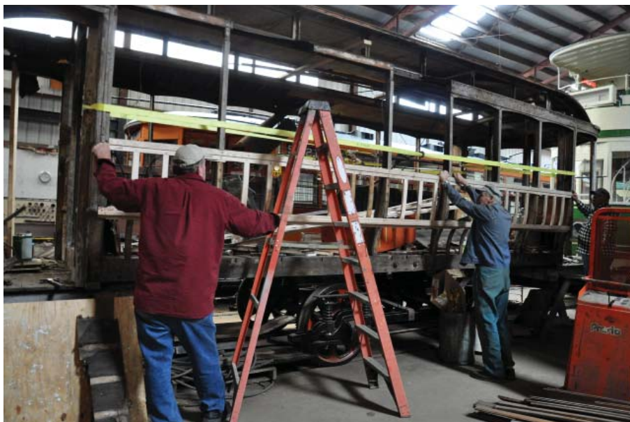
Above: Jim Mackell, Dann Chamberlin, and Dick Avy fit a new belt rail on Lexington & Boston 41, filling voids where doors had been cut in the side when it became a diner. Right: Randy Leclair examines original striping discovered during disassembly. DC
