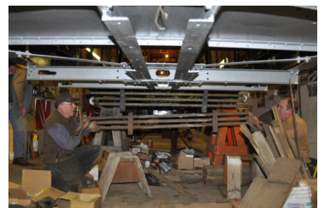
Below: Donald Curry and Gary Anderson position the compressed air radiator under 6131. DC
