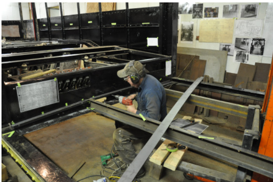
Below: Project Manager Donald Curry drills a hole in the new steel framing that makes up the drop center on Boston 6131. The ABPC automatic acceleration control is mounted just in front of him. DC
