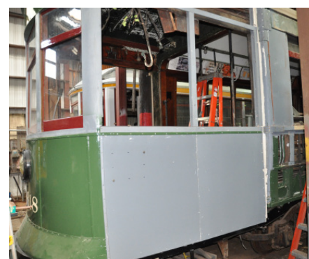
Above: The front platform of 6618, cured of its long-present sag, goes back together.
