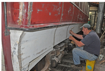
Above: Boston Elevated 25-foot box car 396 showing the restoration work done on the sides and window sash. Repainting is in progress on Philadelphia PCC 2709, just behind 396. JS Right: Jim Mackell removes reinforcing strips from 396 in preparation for repairs and paint. DC
