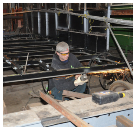
Left: Paul Tetrault and Bernie Bisnette fit a new cross beam in Eastern Massachusetts Street Railway 7005, replacing a badly corroded original. DC Above: John Melanson smooths a weld on the new cross member. The car is of the weight-saving "lightweight" design that saved energy cost and track wear but was subject to corrosion. DC
