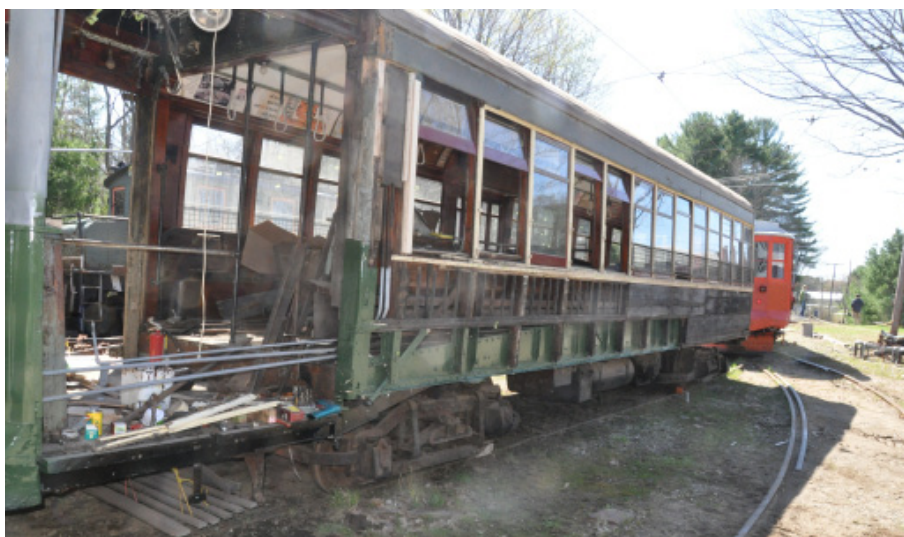
Above: Philadelphia Nearside 6618 being shifted outside the shop. The extensive repair work to the side structure and the front platform are clearly in evidence on this nearly 100 year old classic car. DC
