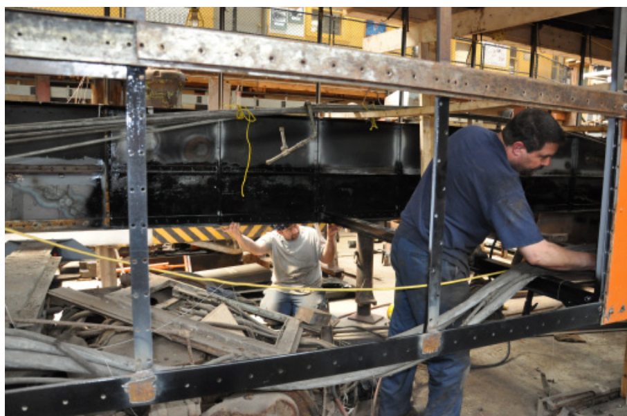
Left: Paul Tetrault and Bernie Bisnette fit a new cross beam in Eastern Massachusetts Street Railway 7005, replacing a badly corroded original. DC Above: John Melanson smooths a weld on the new cross member. The car is of the weight-saving "lightweight" design that saved energy cost and track wear but was subject to corrosion. DC
