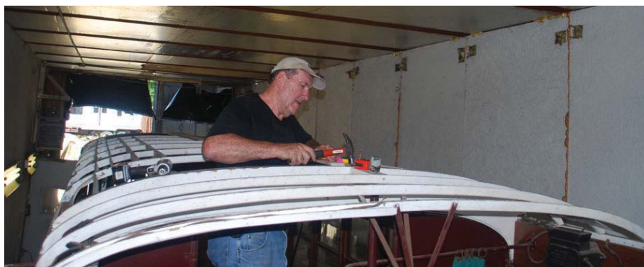
Above: Master woodworker Jim Mackell fastens newly formed roof ribs to Denver Birney No. 1. The car is receiving extensive steel structural repairs in addition to the roof and interior refurbishing. DC
