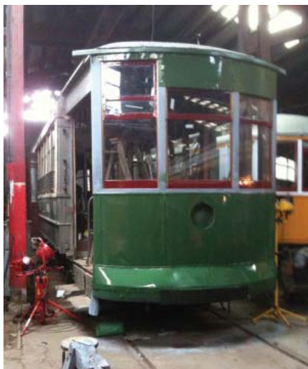
Above: Bob Reich applies glazing putty to a window from Philadelphia Nearside 6618. DC Below: Philadelphia 6618 as it appears after extensive rebuilding of the front vestibule. JS
