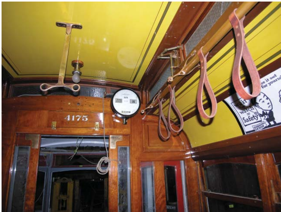
Above: The very careful and thorough restoration of Bay State Street Railway 4175 continued in 2009 as many finishing details including fare registers, hand straps, and many brass fittings were installed. DC
