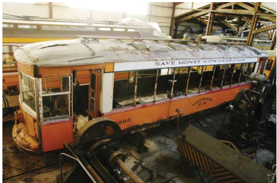
Above: The massive restoration of Eastern Massachusetts Street Railway lightweight car 7005 was launched in 2009 focusing initially on rebuilding the extensively corroded steel structure.
