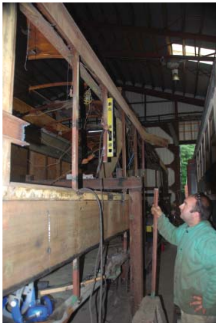
Above: Shop steelworking specialist Paul Te-tault uses a level to position a replacement T-post on Rochester Peter Witt 1213. DC
