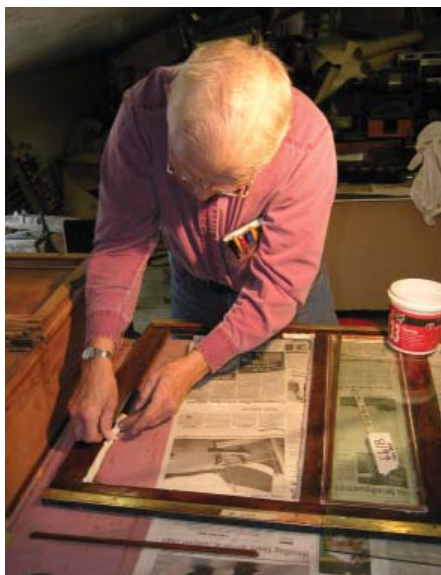
Above: Bob Reich applies glazing putty to a window from Philadelphia Nearside 6618. DC Below: Philadelphia 6618 as it appears after extensive rebuilding of the front vestibule. JS
