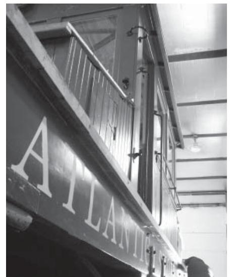
Above: A closeup of lettering just applied to ASL 100. Computer software is used to recreate and scale the lettering based on dimensions of the car and close study of period photos. PM
