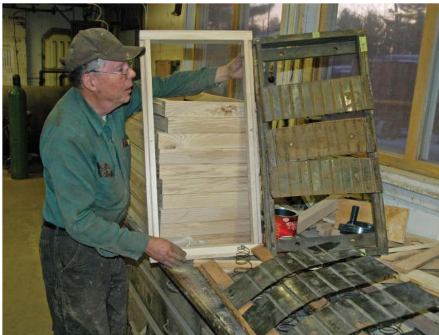
Above: Donald Curry compares a new seat frame for San Francisco Muni No. 1 to one of the 1912 originals. New springs, both coil and flat, are also being fabricated as part of the project. JS
