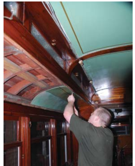
Above: Restoration technician Chris Skulski installs headlining panels in Connecticut 1160. DC
