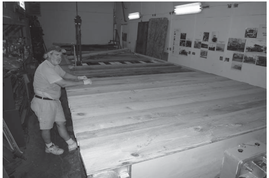
Above: Project Manager Phil Morse pauses while working on installing decking on Atlantic Shore Line locomotive 100. Having been built in 1906, the car predated the widespread use of structural steel. Thus to ensure strength to pull a train of railroad cars, massive wood parts were used throughout. DC
