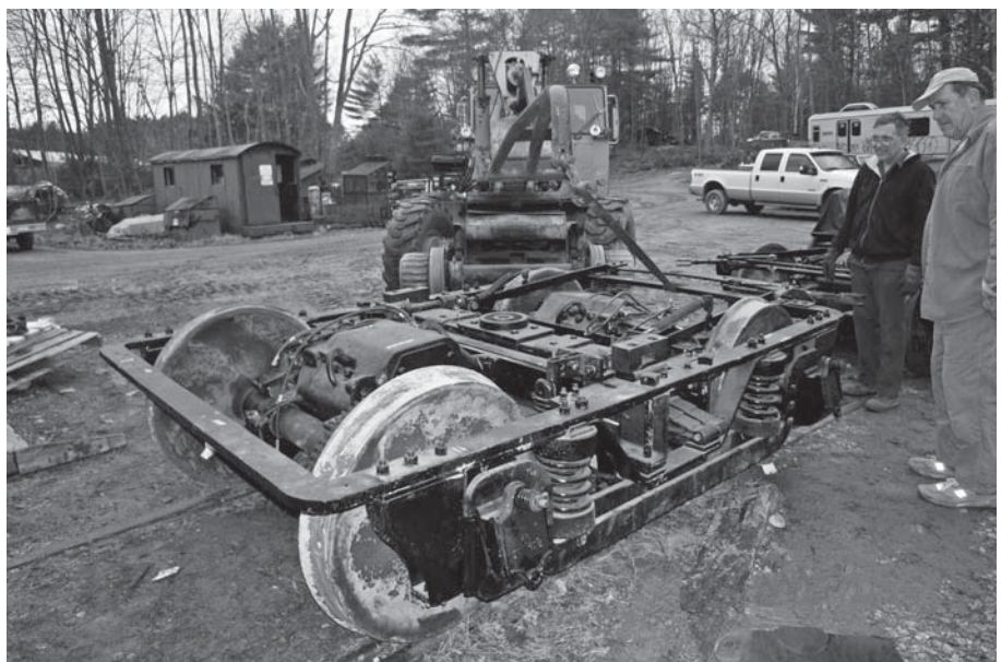
Above: Dean Look and Jim Mackell look on as one of ASL 100's trucks is moved back toward the shop building after its newly overhauled motors have been placed in the truck and carefully aligned with the axles and bull gears. Once inside the shop bearings will be carefully fitted—after being precisely machined. Then gear cases and remaining parts will be reinstalled before they are put under the car. DC
