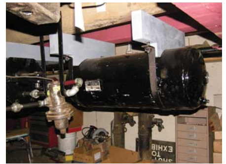
Above: A reconditioned air tank is newly installed under Atlantic Shore Line 100.
