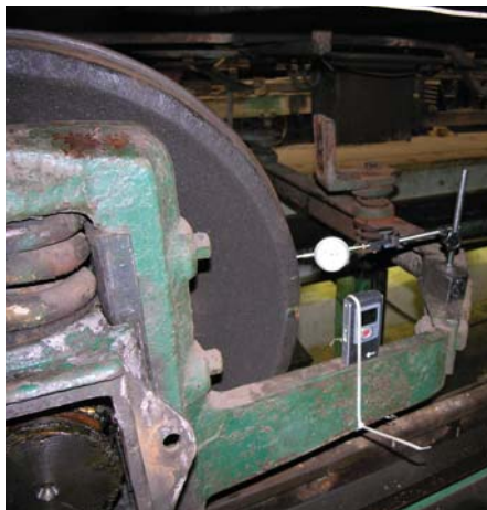
Above: A dial indicator and miniature camera being used to find an out-of-round spot on a wheel from Montreal Observation car 2.
