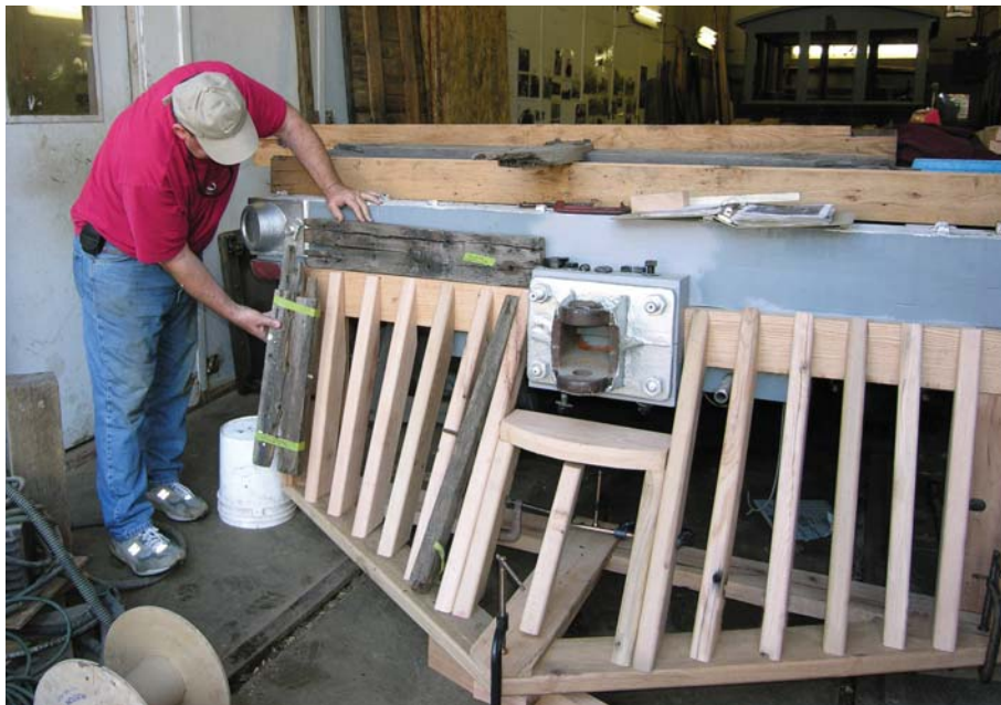
Above: Jim Mackell compares original beams from ASL 100's pilot to the new parts he fabricated. DC
