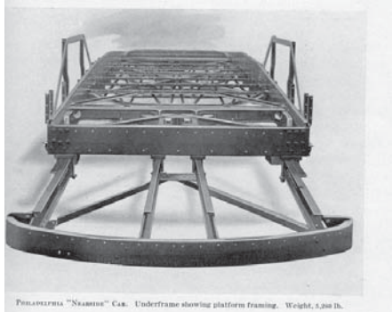
Philadelphia "Nearside" Car. Underframe showing platform framing. Weight, 5,000 lb.
