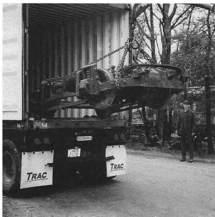
Above: One of the Brill 39-E "Maximum Traction" trucks from Japan is unloaded on arrival. PM
