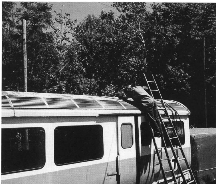
Above: Sliding door mechanism from New York subway car 3352 served as a pattern for the Gomaco Trolley Company who made news mechanisms for Lowell replica 4131 its prototype at Seashore, Eastern Massachusetts Street Railway semiconvertibel 4175. DC Left: Project sponsor Bill Pollman makes steel repairs to the roof of one of Seashore's pair of 01100 series elevated cars from Boston's Orange Line. The cars were built by Pullman in 1957. DC Below: Dan Cohen and Bill Pollman assemble rack shelving in the Parts Warehouse to support pallette storage of motors and other large components. The shelving was obtained second hand. JS
