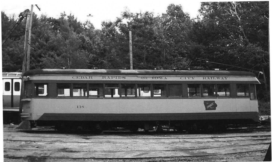
Above: A side profile of CRANDIC 118 shows the lettering and the Iowa-shaped logo. The car was one of the most advanced interurbans built, and boasted a top speed of over 80 miles per hour. JS
