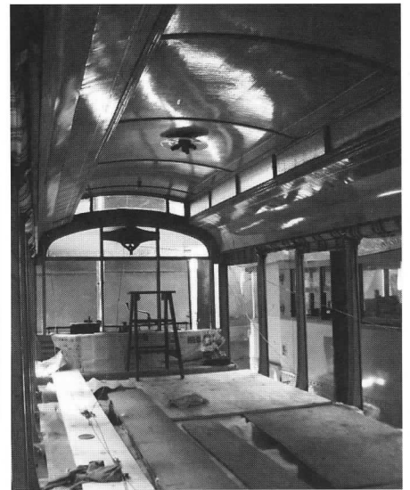
Above: Chris Perry steam cleans one of B&S car 31's Brill 22-E trucks. Right: The car's interior with the seat backs removed to enable refinishing of the natural wood surfaces. DC/JS
