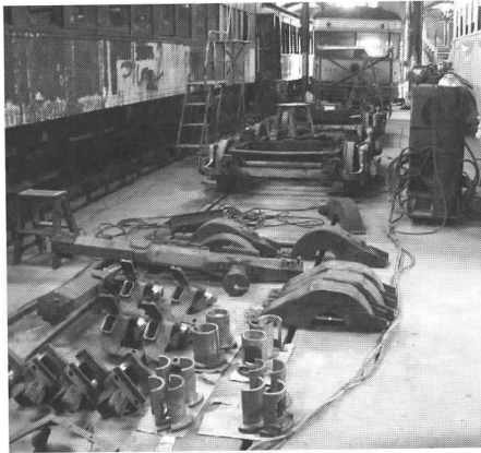
Above: Member Otto Petsch, who has been a valuable source of historical detail, aboard a sister of Cleveland 1227 in the 1940s. Left upper: The car's trucks disassembled during restoration. Left middle: New side bearing plates machined in the shop await installation. Left lower: Veteran signmaker Ken Haselton lays out a destination sign for 1227. OP/JS/DC/JS
