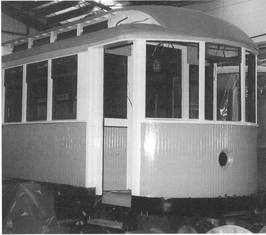
Connecticut No. 1160 shows major progress. Left: Finish colors are on much of the exterior, after extensive refurbishing of the matchboard sides. Above: One of the car's controllers recently reinstalled with all-new wiring. RS
