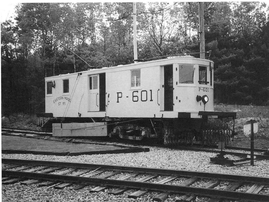
Below: Street railway companies employed specialized cars for snow fighting. Eastern Massachusetts Street Railway P-601 is a snow sweeper with powerful rotating brooms plus wing blades to clear both the track and the adjoining road surface. FM
