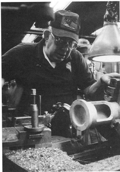
Chicago 225 progress. Left: Chuck Griffith files a newly babbitted motor axle bearing. Center: Shop machinist Ed Johnson expertly turns a motor armature bearing. Below: Ken Haselton applies the distinctive silver Chicago Surface Lines logo to the side of the car. DC
