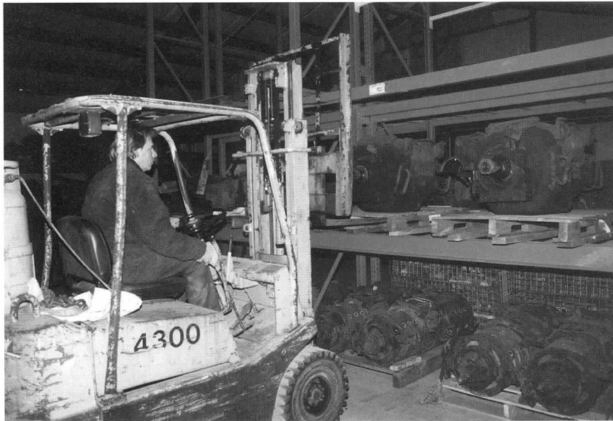
Above: After completion of construction of the Parts Warehouse in 1997, work began in earnest to store large and valuable parts on shelving obtained and installed by volunteers. Here Bill Pollman uses a forklift to place a traction motor on the newly-erected storage racks. DC
