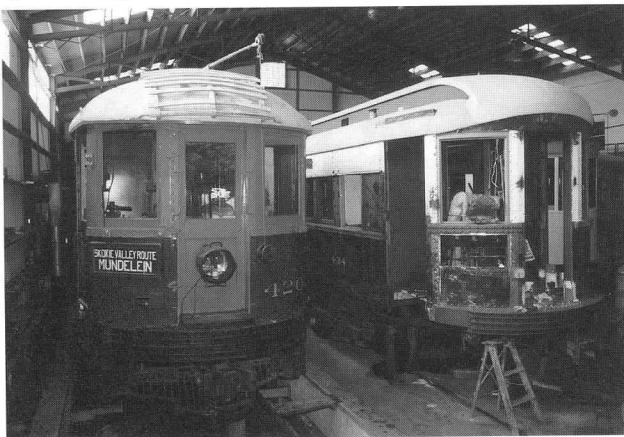
Above: Two Chicago area interurban cars are shown in the shop at the same time. At left, No. 420, from the Chicago, North Shore & Milwaukee is in for routine service. To the right, No. 434, from the Chicago, Aurora & Elgin is undergoing a full restoration program. FM
