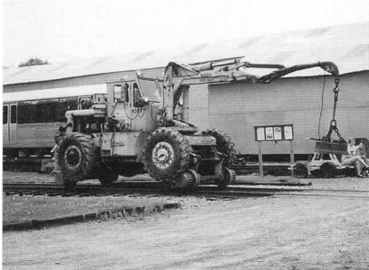
Above: Useful tool for track and signal projects is this high-rail tractor, from Boston's MBTA, shown here equipped with a magnet. FM
