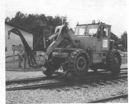
Below: Also useful, and very versatile, is this Pettibone Speed-Swing with Road-Railers. FM
