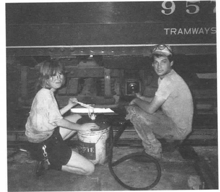
Above: Annie Cooney and Wayne Slayton lubricate the journal bearings of Montreal 957 during annual maintenance in the shop. FM Left: Lisa Alpers carefully reassembles a K controller for Connecticut open 303 after a thorough reconditioning of all its parts. DC
