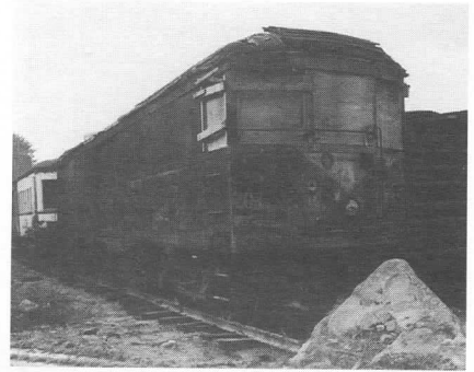
Above: Cincinnati & Lake Erie freight motor 648 is shown behind the shop just before work began on replacement of its roof, the first step in its long-term restoration. By year-end, new roof frame members had been fabricated and installed, and roof boards had been milled. DC Left: Restoration volunteer Amy Litchfield, a year-round regular in the shop, applies finishing touches to the side of Connecticut 1160, readying it for final refinishing. FM
