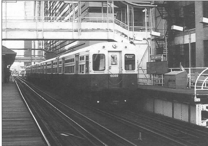
A train of Chicago 6000-series cars, similar to Seashore's Nos. 6599 and 6600, are shown on the famed elevated "Loop," from which the city's downtown district draws its name. The cars were built in the mid-1950's using parts from PCC streetcars. WP
