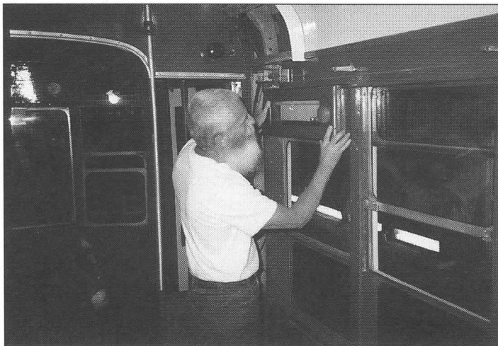
Left: Shop crew member Richard T. Lane, Jr. installs one of 631's destination sign boxes, a feature removed during the car's years in Vienna. FM
