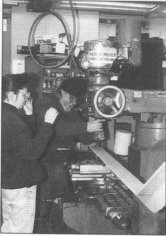
Liz Cooney watches as Shop Crew member Bob Webb machines new platform knees for Connecticut 1160. DC
