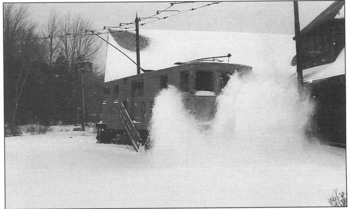
Eastern Mass. snow sweeper P-601 demonstrates with its whirling brooms some of what would be needed if Seashore were to operate in the winter months. DC
