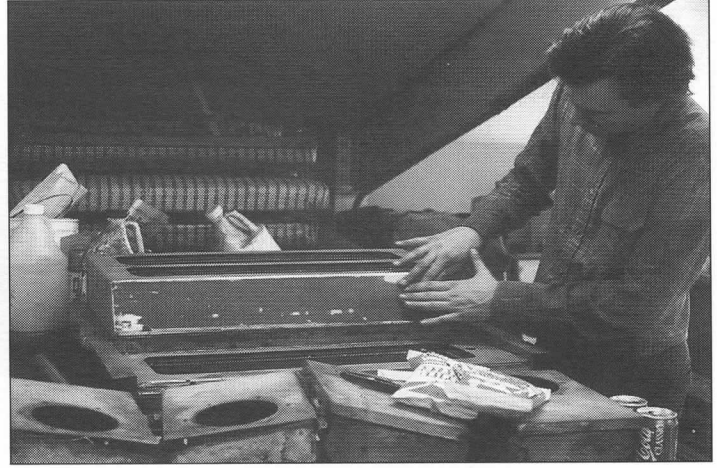
Other components from the cars receiving repairs were the sign boxes and marker light boxes, shown here in the second floor loft of Town House Shop. DC
