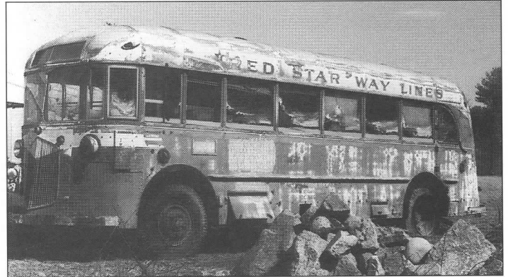
Added to Seashore's rubber-tired fleet in 1994 was this interesting 1934 streamlined interurban bus. The Model 23S Twin Coach once served in St. Clairsville, Ohio. RK
