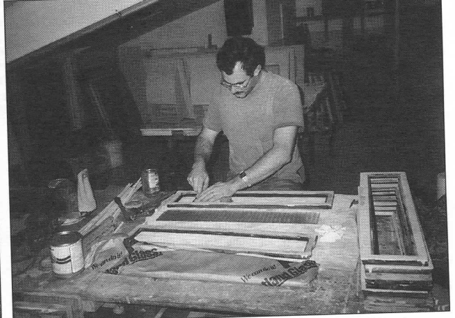
Above: Proper restoration of window sash requires removal of the glass, stripping and repairing wood frames, refinishing, then reinstallation of glass. Here Stephen Santarelli reglazes clerestory sash from Bay State 4175. FM Left: When Bay State 4175 was modernized, interior bulkheads were removed. In this view, shop woodworking specialist John Mazzei sands the surface of one of the intricate new bulkheads he fabricated for the car. DC
