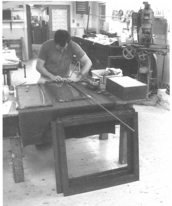
One of the most labor intensive parts of any early streetcar is treatment of the windows and doors. Steps involved include stripping old finishes, disassembly, repair or replacement of damaged wood, refinishing, and glazing. Here Project Sponsor Stephen Santarelli glazes upper sash from Bay State 4175. JS
