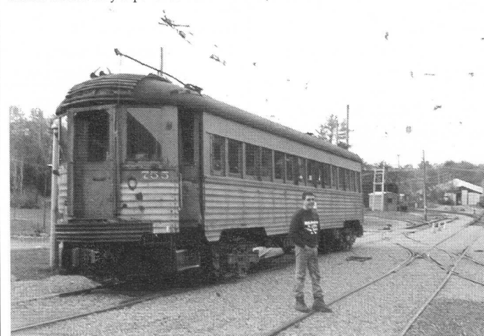
Member Mark Scannell with Chicago, North Shore & Milwaukee interurban 755. These cars demonstrated the great flexibility of electric rail transit as until the early 1960s they began in Milwaukee's city streets, continued south on their own high speed right-of-way, then travelled to Chicago's midtown "Loop" on the tracks of the elevated. TG
