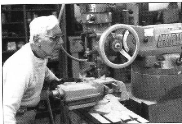
CAR MAINTENANCE: Volunteer Dick Howe expertly fabricates new parts for a controller from Boston rail flat No. 2026 using a vertical milling machine in the restoration shop. JS
