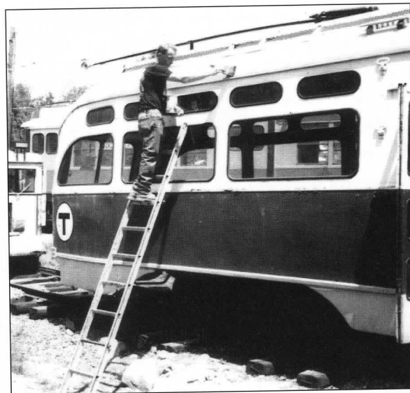
BOSTON MBTA No. 3292: Peter Folger applies fresh coat of gray paint to the roof both to improve the car's appearance and enhance its conservation. FM
