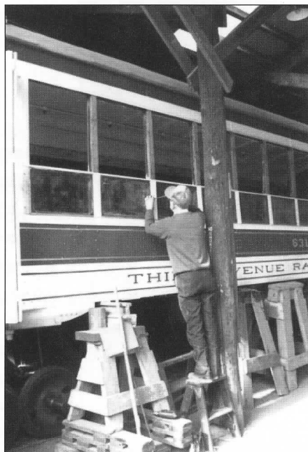
THIRD AVENUE No. 631: Volunteer project sponsor Arthur Duncan prepares the car for repairs to corroded window posts. Note the newly regauged axles waiting under the car. JS
