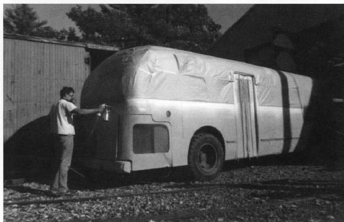
◀ Final colors are sprayed on No. 627 at the rear of the shop. A long term need for the shop is an indoor spray booth.
