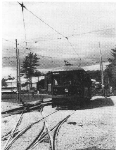
▼ Philadelphia & West Chester No. 62 approaches the double-slip switch in the platform area newly paved with crushed rock. J. Schantz
