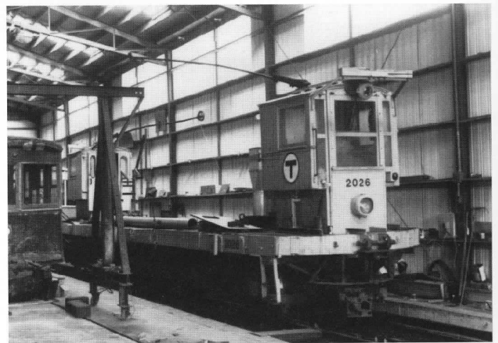
▼ On the repair pit for routine maintenance is Boston rail flat No. 2026, a vital tool around the Museum. The cut-away cabs were designed to allow carrying rail. J. Schantz
