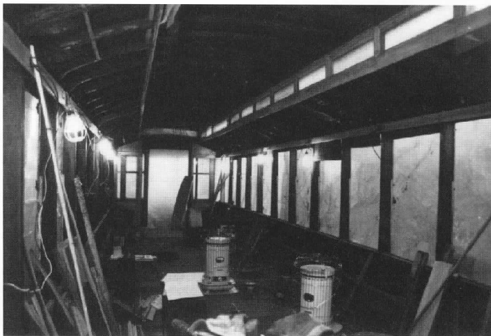
All seats, interior fittings, and woodwork had been removed from Twin Cities Gate Car No. 1267 for refinishing and repair in this winter view. D. Black
