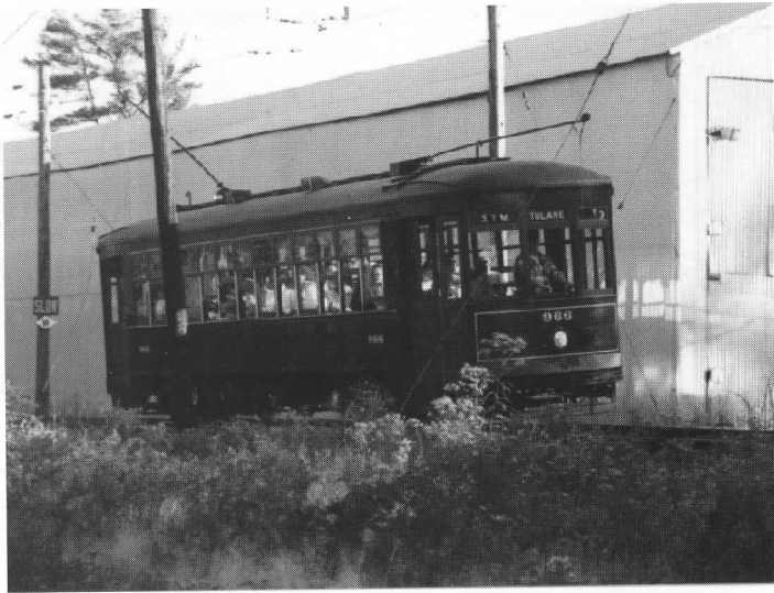
A major event of 1990 was the first operation of New Orleans 966 on the Museum's track. An intensive restoration effort and conversion of the car's trucks from New Orleans broad gauge brought the car to life for the first time since the Canal Street line was abandoned in 1964. D. Black photo
