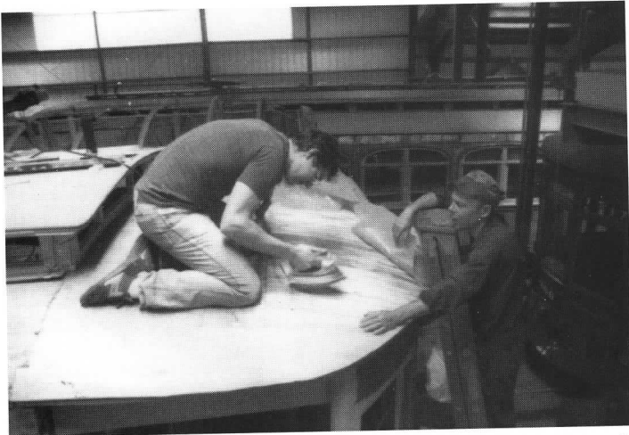
A steam iron is used to correct minor warping prior to final sanding on the bonnet of Bay State 4175. The new roof was complete by year end. B. Austin photo
