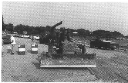
Left: Seashore's newly acquired Caterpillar bulldozer was an important tool for preparation of the unloading area.
