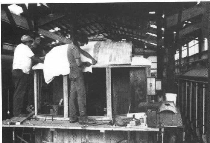
Once roof boards are complete, the canvas is stretched into place and tacked. A combination of volunteers and permanent staff work on Aroostook Valley 70.
