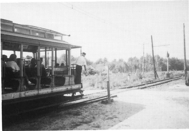
Connecticut Open 303 shown pausing to pick up the staff allowing it to proceed out the main line. Use of the staff is a safety measure adopted in 1989.
