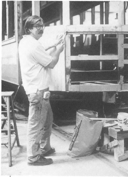
A veteran shop employee carefully installs a new tongue and groove dash on Twin Cities 1267.
