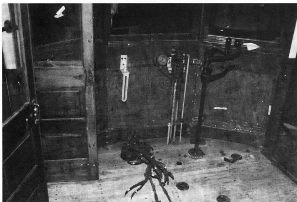
LEFT BELOW: The first platform of 225 shows considerable progress after having been similarly dismantled. Many frame members plus the flooring have been completely replaced. JDS
