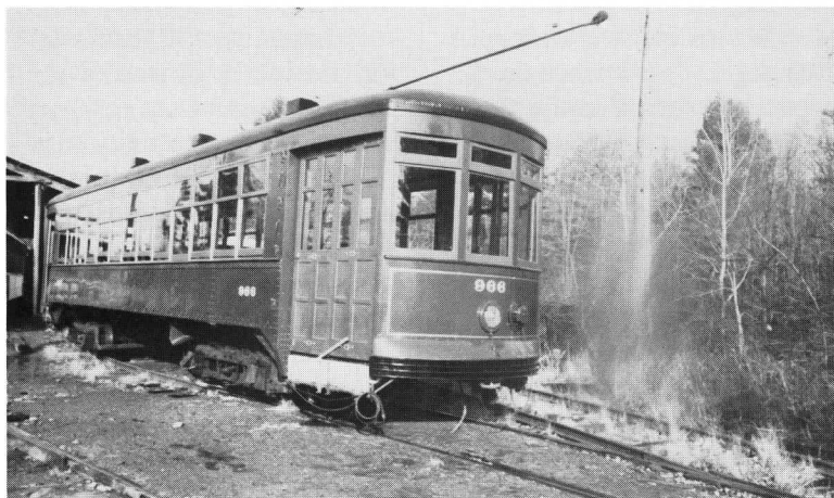
New Orleans 966 received final colors in 1988, but remains on shop trucks pending completion of its own trucks next year. C. PERRY
