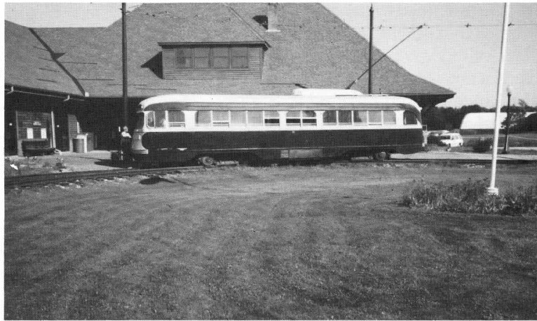
Seashore's first PCC car was Pittsburgh 1440, acquired two decades ago. Re-gauged to operate on standard gauge track, and restored inside and out, the car is shown here in front of the Visitors Center. F. MALONEY
