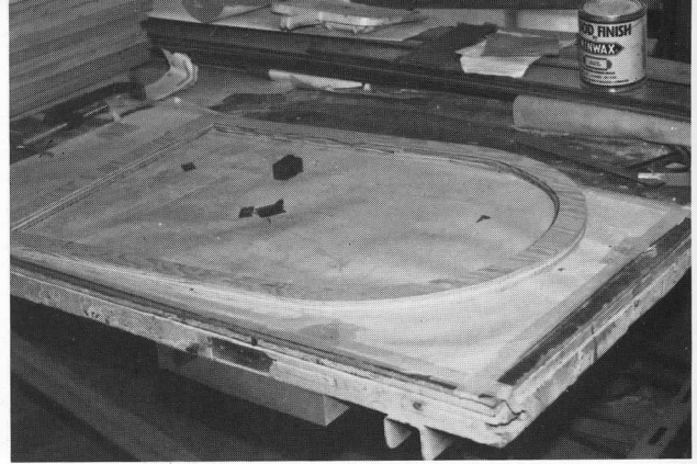
ABOVE - Shop projects in 1986 included fabricating unusual arched window sash for Wheeling 39. A distinctive feature of Cincinnati curved-sides was such windows with the semi-circular top located in the panel over the sliding door pockets. FRED PERRY
