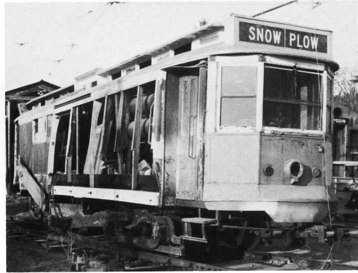
No. 3 Semi Snow Plow 5164 once again mobile after total replacement of a composite wood and steal side frame. TSDeB
