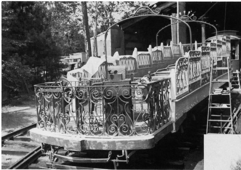
1. Montreal observation Car No. 2, shown undergoing complete exterior re-painting. Still to be done is the refinishing and reinstallation of the car's seats. One of the only four survivors of what was more of a Canadian institution, the grand stand type of observation car (Cincinnati a rare exception in U.S.). Ours was the donation of Canadian Breweries.
