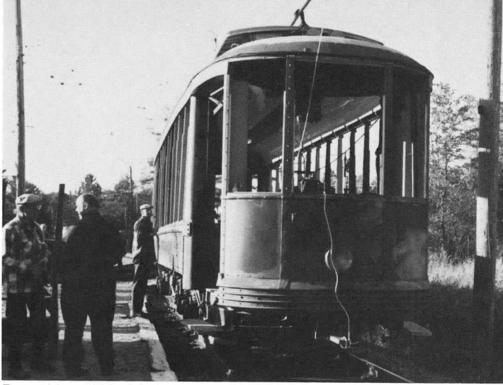
Eastern Mass. 4387's air brake system and piping were reinstalled. The PC-5 control unit, after overhaul, was also reinstalled along with associated wiring. Photo shows car fully operational on Members' Day. TSdeB
