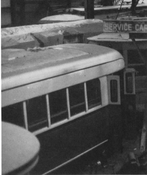
Installation of new roof canvas on Boston PCC car 3127 was virtually complete when this photo was taken. POLLMAN
