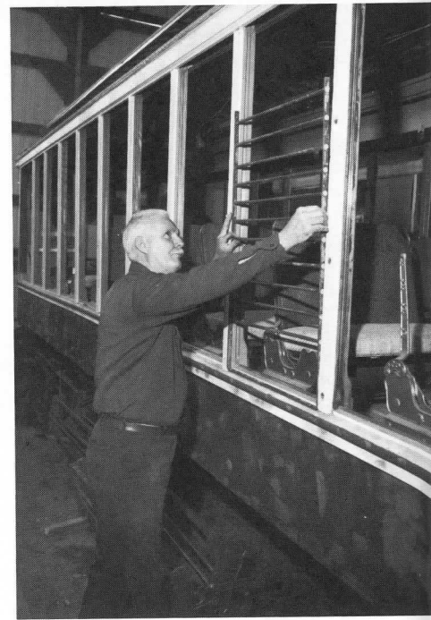
RIGHT — 4547 was acquired by the Museum in work car status with summer time window guards long discarded. A brand new one is being fitted, made by our shop from a blueprint furnished STM by the Branford Electric Railway Association, who have been most helpful in many phases of this restoration project. WOOLNOUGH
