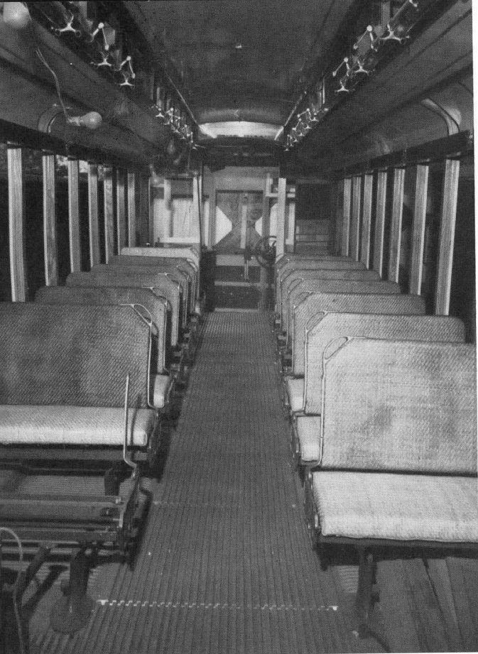
LEFT — Detailed restoration of Brooklyn Rapid Transit 4547's interior continued in 1984. In this era of metal and plastic transit vehicle interiors, 4547's, with its carefully restored brass-trimmed varnished wood, will make it still another "Jewel in the Crown" in the Museum's collection. WOOLNOUGH
