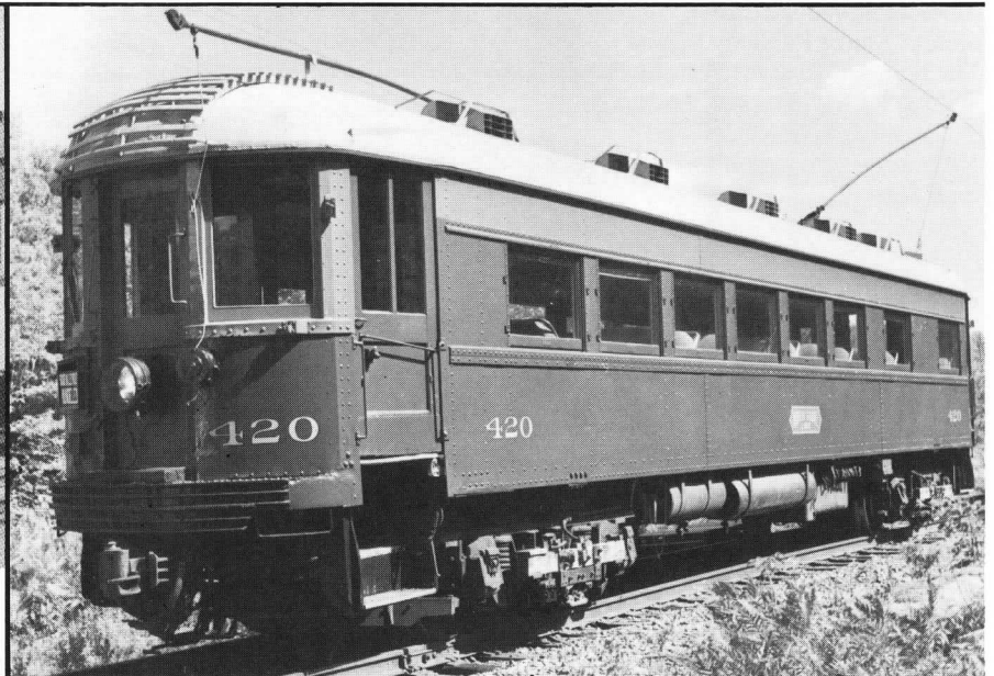
ABOVE RIGHT — Chicago, North Shore & Milwaukee 420 shown after roof and body work that was followed by its repainting with the new IMRON enamel in that road's latter day green and red paint scheme. It contrasts with its appearance when outshopped by Pullman in 1928 as the last and most deluxe of the four observation cars built for the interurban, the only one to be outfitted with swivel armchairs. With the depression setting in shortly thereafter, by 1932 this prestigious parlor car service was eliminated. An added saving was the doing away with the running of trains hauling these single end cars all the way south on the Chicago "L" to 63rd St. to wye them.
