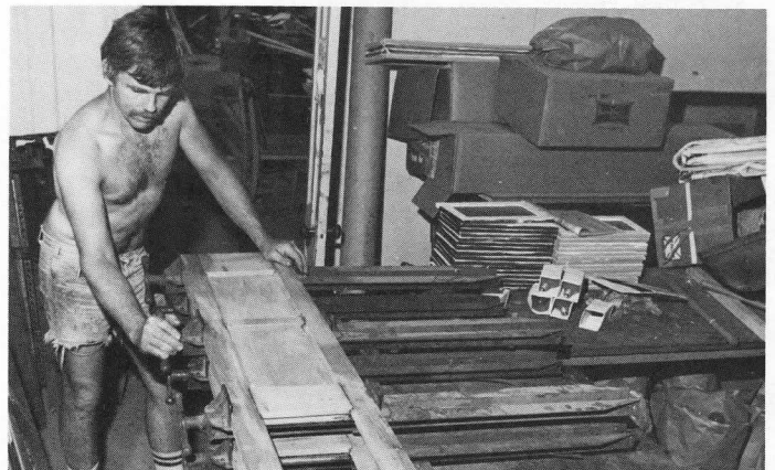
Work progresses on new New Orleans car doors for two museums.
