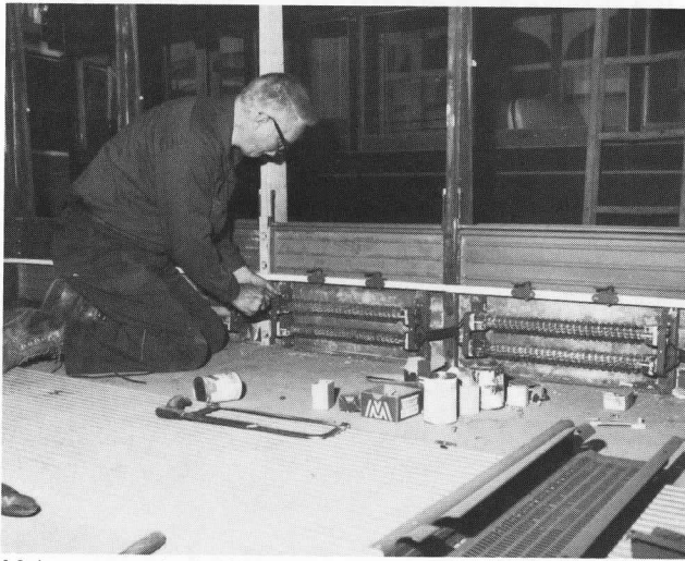
Major structural rebuilding of cars requires painstaking reassembly of inside finish, seats and as many as five electrical circuits, to say nothing of repiping air brakes systems. LEFT — Don Gawthrop putting back Eastern Mass. 4387's heaters. RIGHT — A volunteer fastening down motorman's floor matting in south vestibule of 4387. WOOLNOUGH TSdeB
