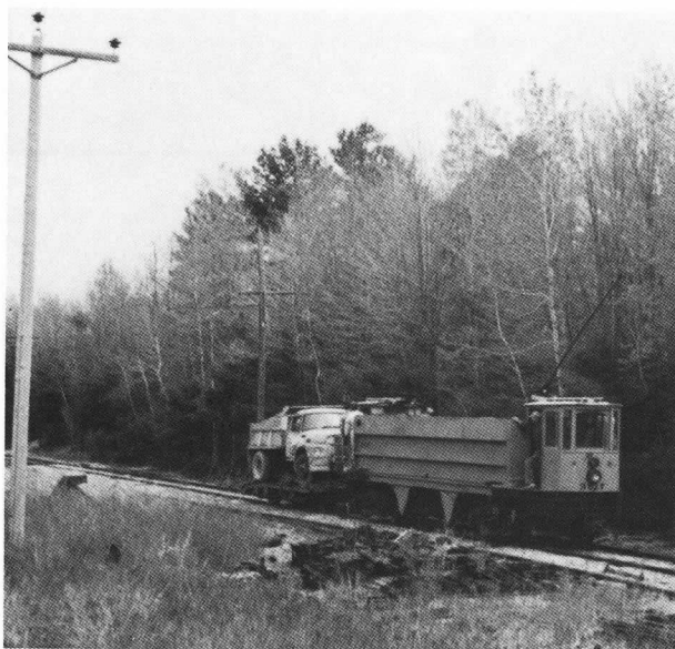
Bottom Dump car 3617 pulling ramp car with dump truck aboard, a frequently used combination for off-track grading, filling and ballasting operations. R. T. Lane
