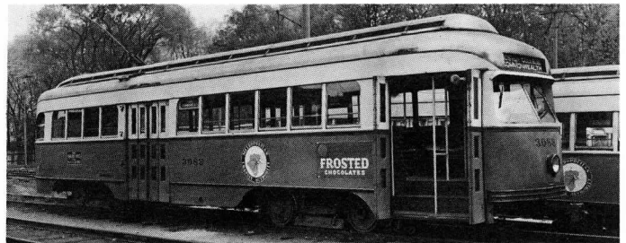
P.C.C. car 3083 equipped by M.T.A. with Railvane fans and "monitor" roof poses at Reservoir carhouse. CHENEY
