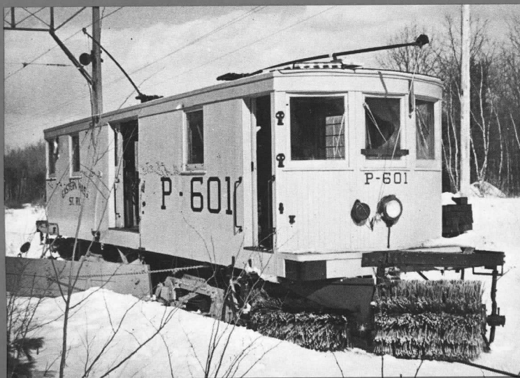
Sweeper P-601 clearing the "Rochester, Syracuse and Eastern" section of the main line after a brief return to shop for rebuilding of brooms and repairs to driving mechanism. RS&E once had a similar Russell sweeper. WOOLNOUGH
