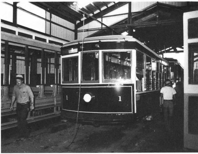
Work was being rushed on Birney No. 1 to have it ready to run on Members Day. With most electrical, mechanical and body work complete, there remained many leaks to be fixed in the complex safety car air system.
