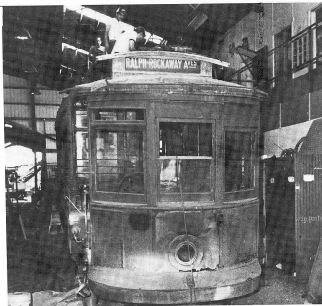
4547 before dismantling of vestibules — a step necessitated by the need for rebuilding of platform knees and the underframe of the body of the car as well.
