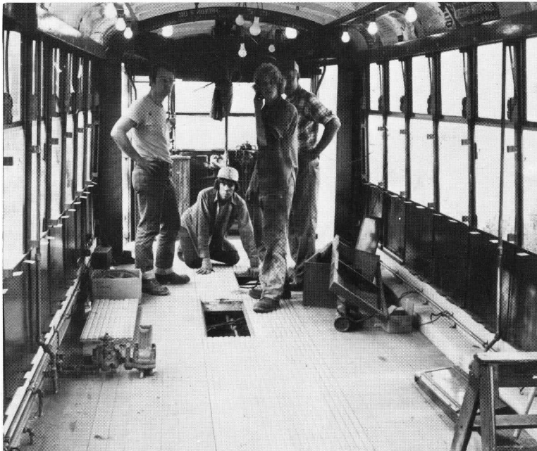
After. Photo taken near end of season, 1979. Shows basic work completed on sides of No. 5821. Although still minus window sash, doors, seats and inside trim, car had already been re-equipped electrically and mechanically. At this moment it is being readied for a trial run on the main line on Member's Day. Woolnough Photo
