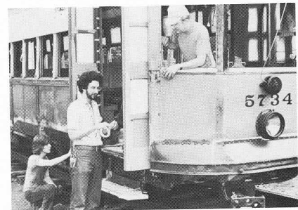
Boston area museum volunteers engaged in three week crash program taking Type 5 No. 5734 out of the "mothball fleet" and readying it for its return to Boston for the Highland Branch's Twentieth. Woolnough Photo
