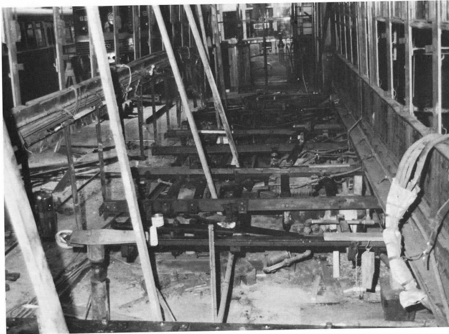
Before. Photo taken in mid-summer 1978 contrasts sharply with photo on opposite page. Boston Type 5 Semi No. 5821 as it appeared with major portions of the underframe renewed and side "T" posts on the first side rebuilt, in readiness for riveting on of new side sheets. Woolnough Photo
