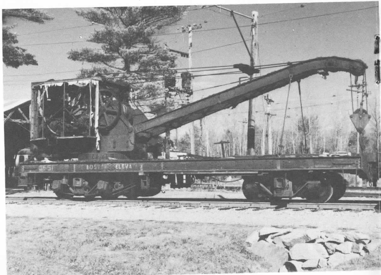
Former Red Line Crane Car No. 0551 shortly after its arrival from MBTA's Cabot Maintenance Center. With greater lifting capacity than 3246 and equipped with MCB wheels, it should shortly prove its usefulness in the Shop and elsewhere. — Woolnough.
