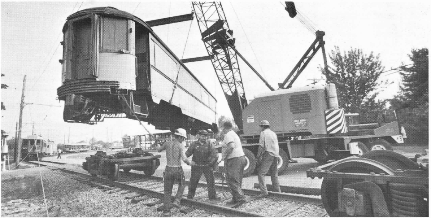
North Shore Line Diner 415 finally arrives at Seashore after several years of negotiations. C.N.S. & M. #420 stands by in background to tow reassembled car away to shops for reconnecting brake rigging — Hanlon
