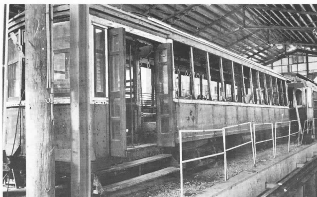
Montreal No. 957 as it appeared during the early stage of its restoration. The side window sash and interior trim have been removed for repair and refinishing. The roof has been stripped for rehabilitation. Brilliant photo.
