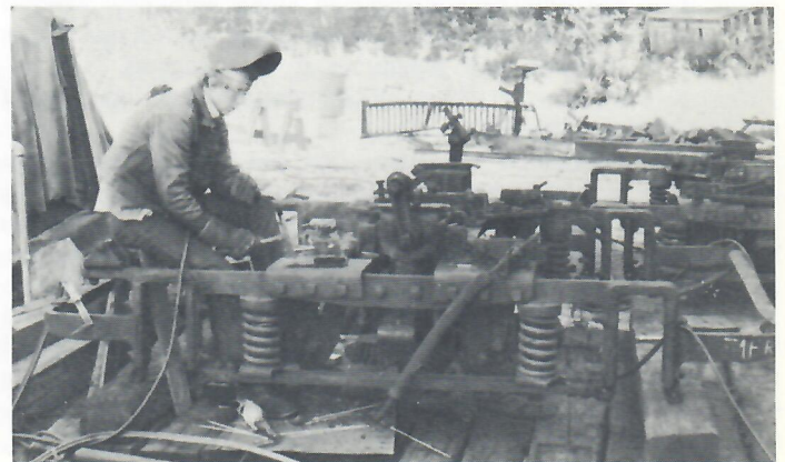
Jim Schantz, spearheading the re-gaging of 62's trucks at work cutting out necessary pieces of metal to correctly position brake rigging for standard gauge. (Tibbets Photo)
