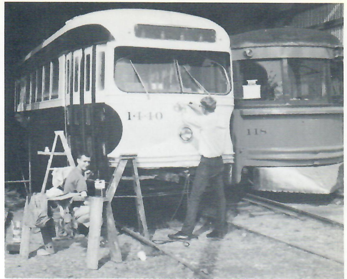
1440 — Pittsburgh P.C.C. built by St. Louis was only new street car to be added to Seashore collection in 1968. It is shown here receiving finishing touches of vermilion and cream restoring it to an earlier paint scheme. Still on shop trucks, regauging must wait until standard gauge Clark B-2 truck frames can be obtained. (Santarelli photo)
