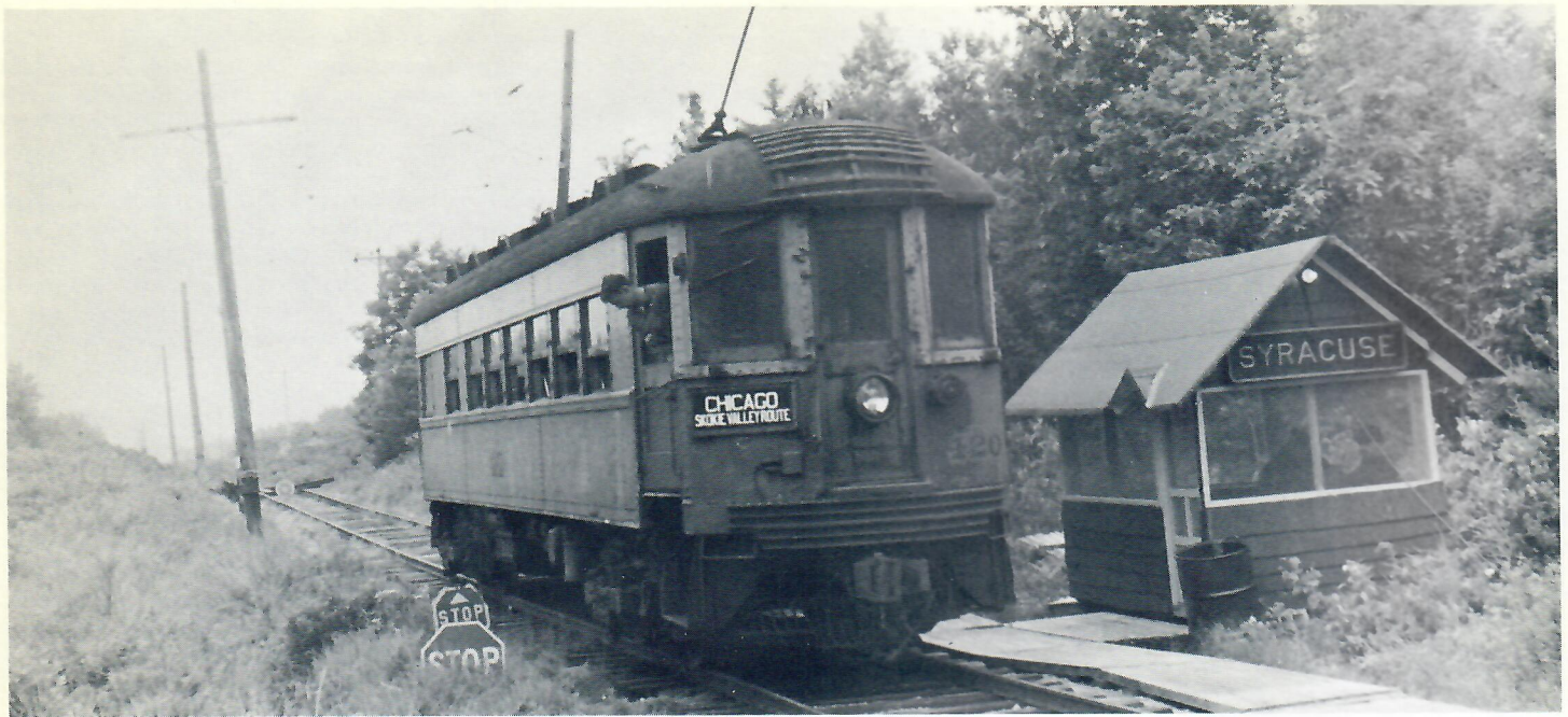
North Shore Line #420 shown on one of its first trips out on Seashore's Main Line after arrival. To the right is Syracuse Sta. marking temporary end of line and sporting sign from old NYC station in Syracuse, N.Y. This end of #420 was originally the observation end with brass railing and canvas awning when outshopped by Pullman in 1928. It was converted to coach and motorized with two motors salvaged from Merchandise Dispatch cars during World War II. (Munroe photo)
