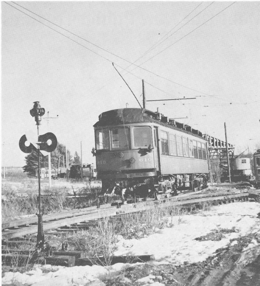
View, looking south on main line at "Doherty" switch, with M&SC 610 in the foreground. Note the Lehigh Valley switch stand controlling lead to Riverside barn. (Munroe photo.)
