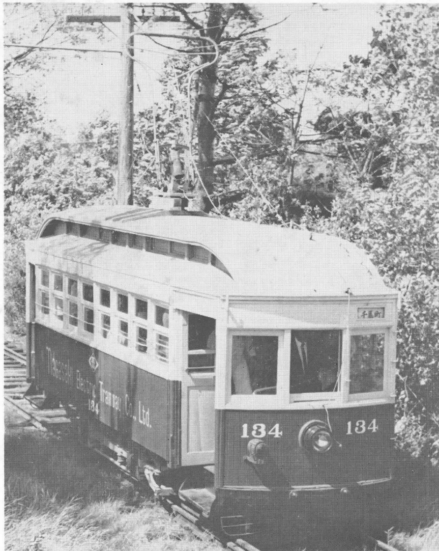
Nagasaki (Japan) Street Car No. 134 was being demonstrated to some of the many guests that attended the presentation ceremony when this photo was taken on June 25th. Scene is just north of Clough's Crossing on the main line. Note the bow trolley. The car was shipped via the United States Lines aboard the Pioneer Minx. (Shelvey Photo.)
